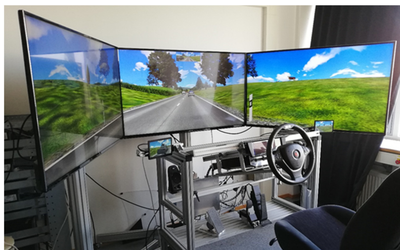
Figure 3. Structure of the static driving simulator.
