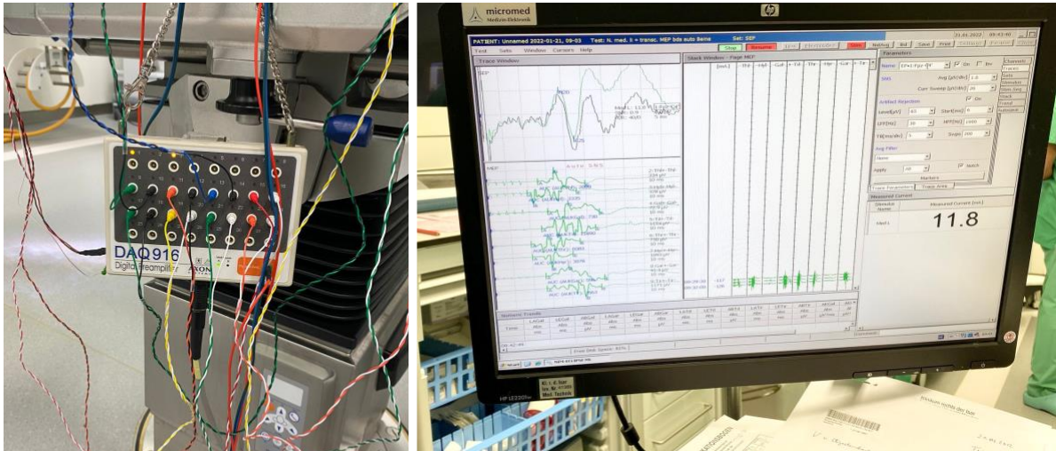
Figure 11: Intraoperative Neuromonitoring Unit.
