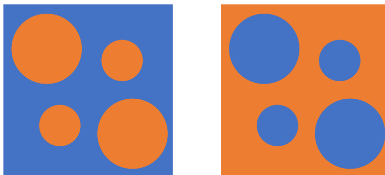
Figure 2.10.: Illustration of scattering contrast. X-ray and neutron scattering detects interfaces arising from a contrast variation |\Delta|^2 and do not directly relate domains to a certain SLD . According to Babinet's principle, scattering from an 'orange' domain in a 'blue' matrix yields the same intensity pattern as scattering from a 'blue' domain in an 'orange' matrix.
