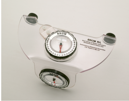
(a) Back Range of Motion Instrument (BROM) with a compass goniometer (upper part) and a gravity inclinometer (lower part).
