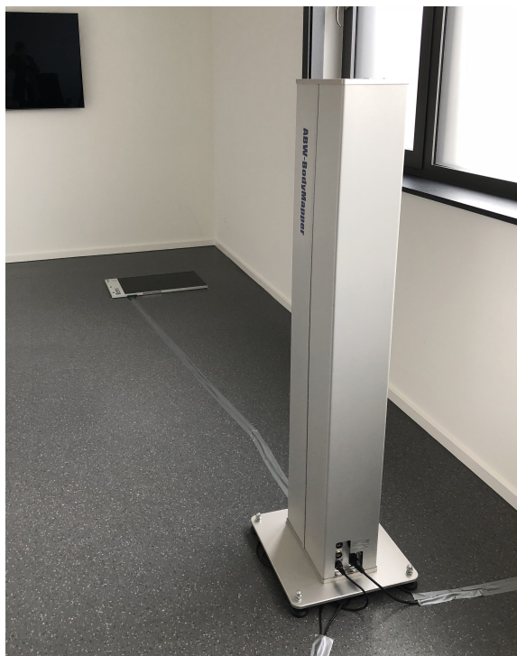
Figure 2.5: Set-up for static alignment and pedobarography assessment.
