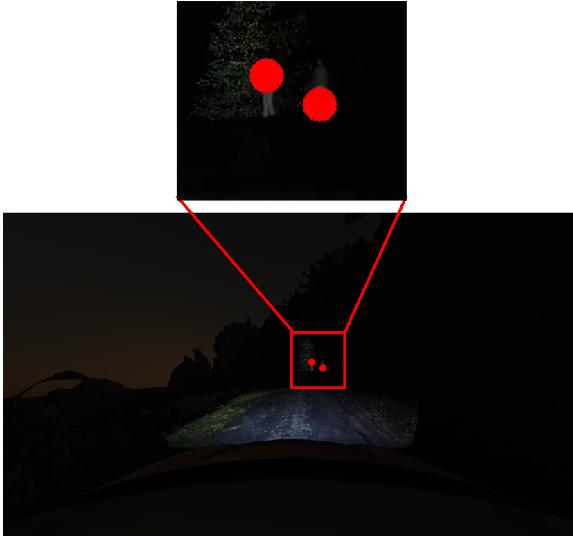
Figure 7.9: Spectators during nighttime: The red circles illustrate the RADAR detections.
