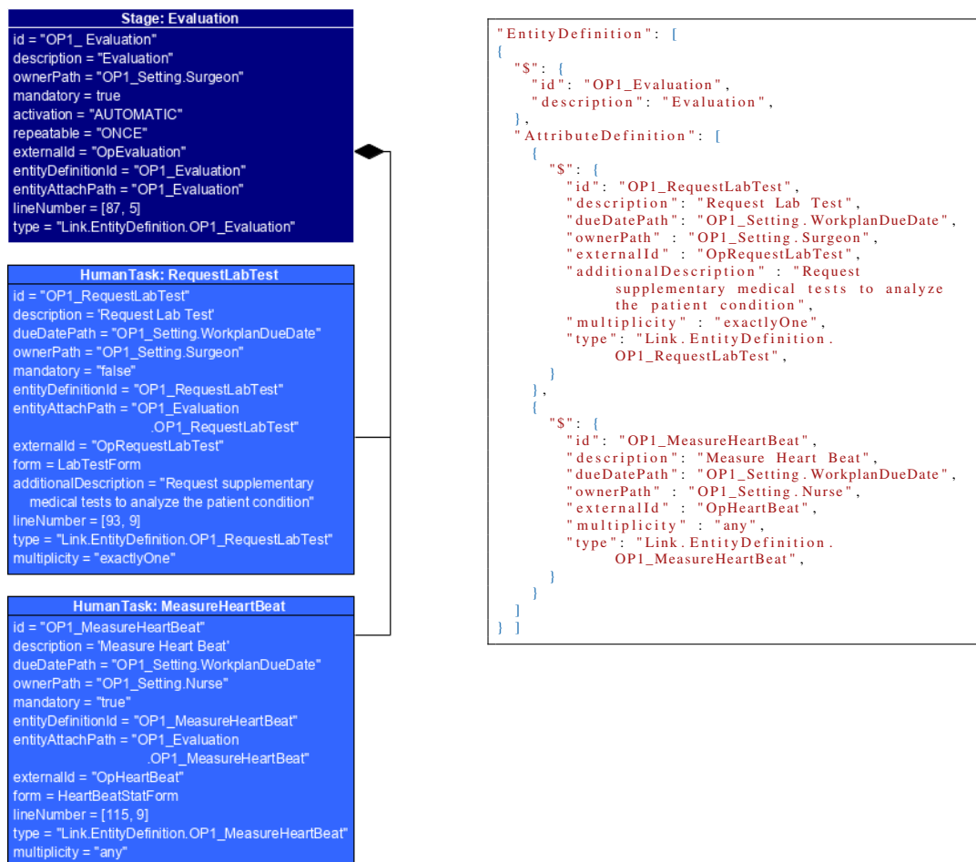
Figure 6.13: Example of compiling a interpreted Stage (left) into SACM JSON structure of EntityDefinition (right). The Attribute-related properties of HumanTasks in the Stage constitute their AttributeDefinitions.
