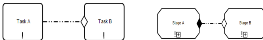
Figure 2.6: CMMN Sentry establishes a dependency between two Tasks (left) or two Stages (right). The white diamond represents an Entry Criterion, while the black diamond denotes an Exit Criterion.
