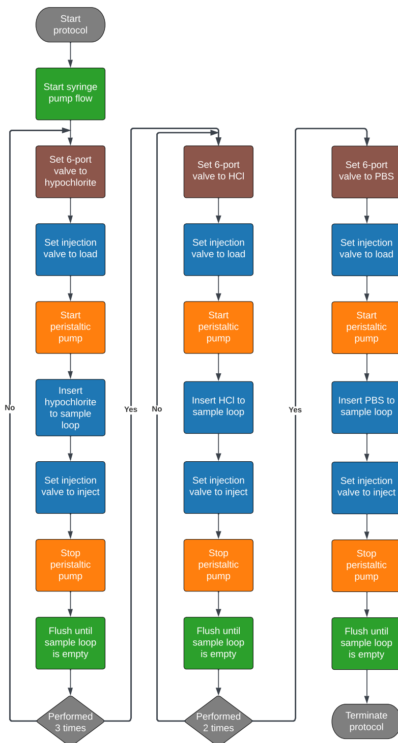
Figure A.2: Flow diagram of the washing protocol. The washing protocol includes three washing steps with 2.5% hypochlorite, two steps with 0.1 mol HCl and one with PBS. Each colour represents a different device.
