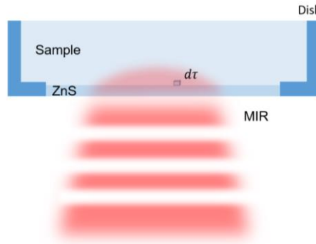
Fig. 3-2. Illumination of MIR beam on the sample. Due to the absorption, the MIR beam exponentially decreases as it penetrates the sample. To simplify the discussion, we take a small volume d\tau that is close to the bottom surface.
