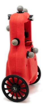
Figure 1.1: TWIP with markers for an optical tracking system
