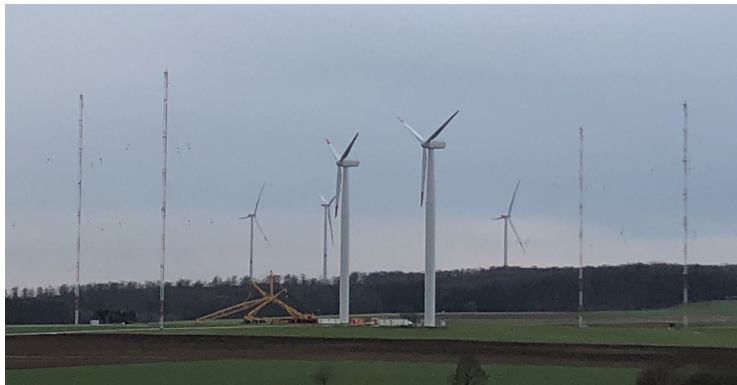
Figure 6.13: Test site with the two turbines and four met masts. Source: ZSW www.zsw-bw.de
