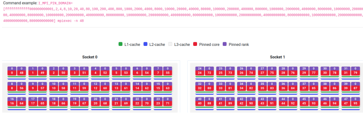
Figure 5.2: Screenshot from the Intel pinning simulator. It shows the pinning used in this work. A computing node on SuperMUC has 48 physical cores and 96 threads (with Hyper-Threading enabled). The first rank has the first thread of core one and thread two of every other core. The other ranks have one thread each. The OpenMP parallel code runs on rank zero, where it can use up to 48 threads.
