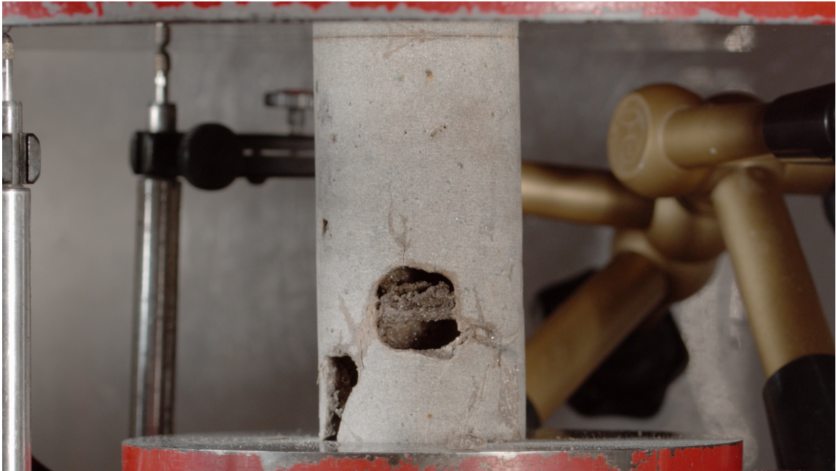
Figure 5.22: Compression test of a core sample. Photo showing the resulting crack.
