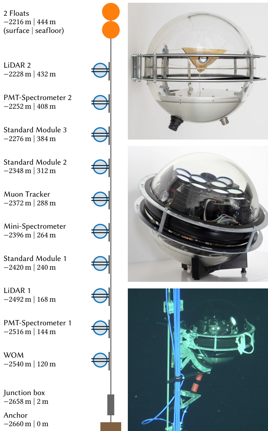
Figure 2.6: Sketch of the STRAW-b mooring line (left) with the position of each module. The Standard Module 3 (upper right) that hosts the art project radioamnion [26] and the PMT-Spectrometer (middle right and lower right [27]) are shown exemplarily.
