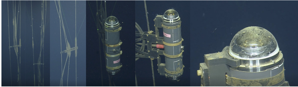
Figure 7.3: Collage of the STRAW inspection from September 2020 operated by Ocean Networks Canada (ONC) [27]. Biofouling appears at the modules and along the cables.
