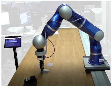
(a) CIP : Autonomous anomaly detection when grasping object.
