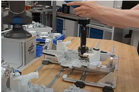
(c) Demonstrating how to insert the motor into the housing.
