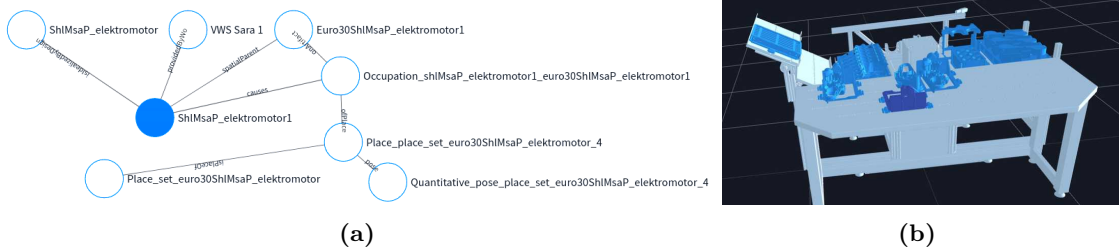
Figure 8.2: Graphical representations of ontological knowledge. (a) shows entities (circles) and their properties (lines) that are modeled in the ontology. The example shows a physical object marked as blue dot ( Artifact ) of a specific type ( \rightarrow idealizedByDesign \rightarrow Design ) and how it is geometrically ( \rightarrow spatialParent \rightarrow Storage ) and semantically ( \rightarrow causes \rightarrow Occupation \rightarrow ofPlace \rightarrow Place ) referenced in the ontology. (b) Visualization of the variable workstation.
