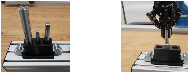
(a) Three different peg-in-hole problems with un-square, small round, and large round peg. The left and right ones are contained in the SVM training set. (b) Exemplary peg-in-hole task with unseen objects.
