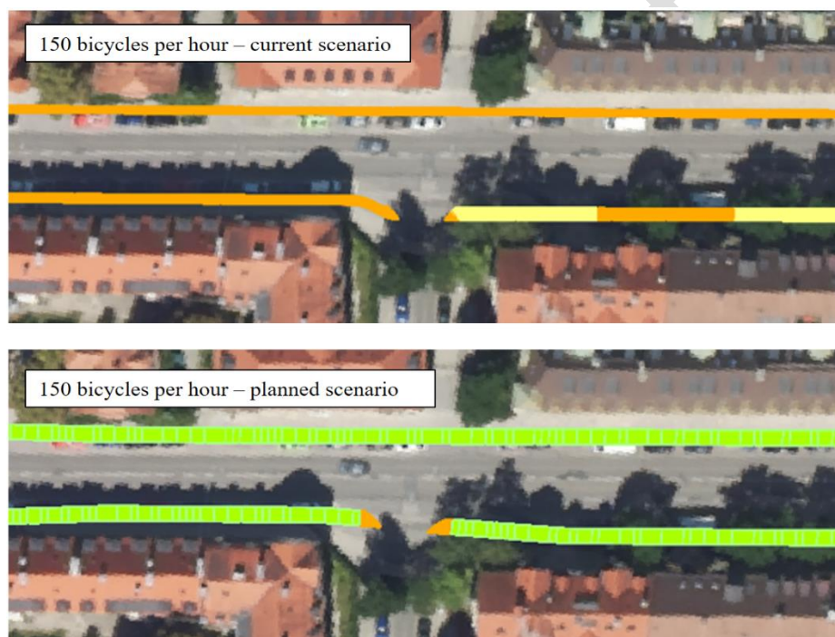
Fig. 5. Comparison of BLOS values at 150 bicycles per hour of the current state of bicycle paths with a planned scenario.
