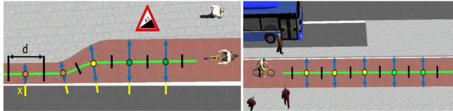
Fig. 2. Width calculation of bicycle paths at short intervals and determining adjacent surfaces.
