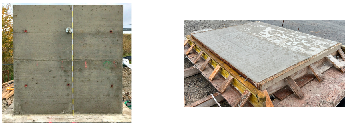
Figure 1. Left: test wall (C4) and right: test slab (C3). Both 2.00 m × 2.00 m × 0.25 m.
