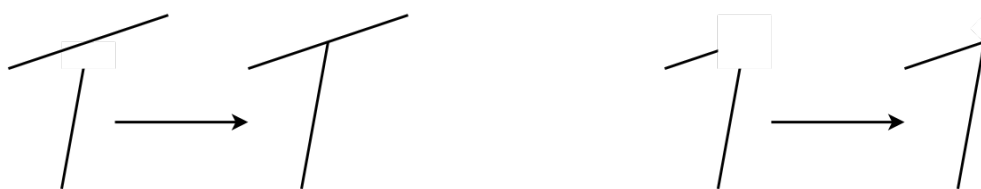
Figure 2: Schematic explanation of the merging of unconnected parts in 2D: Join on passing elements (left) and join of free ends (right)
