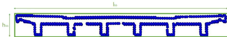
Figure 3.10: An illustration of the bounding box of a point cloud cross section
