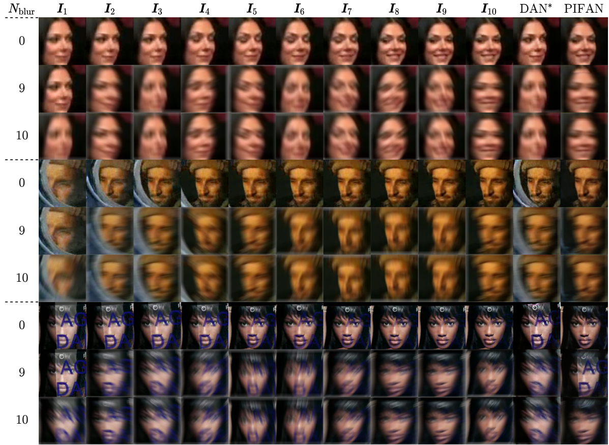
Figure 6.4: Qualitative results for three videos with N = 10 frames. For every video, N_{\text{blur}} \in \{0, 9, 10\} frames are tampered with motion blur of filter size 19.
