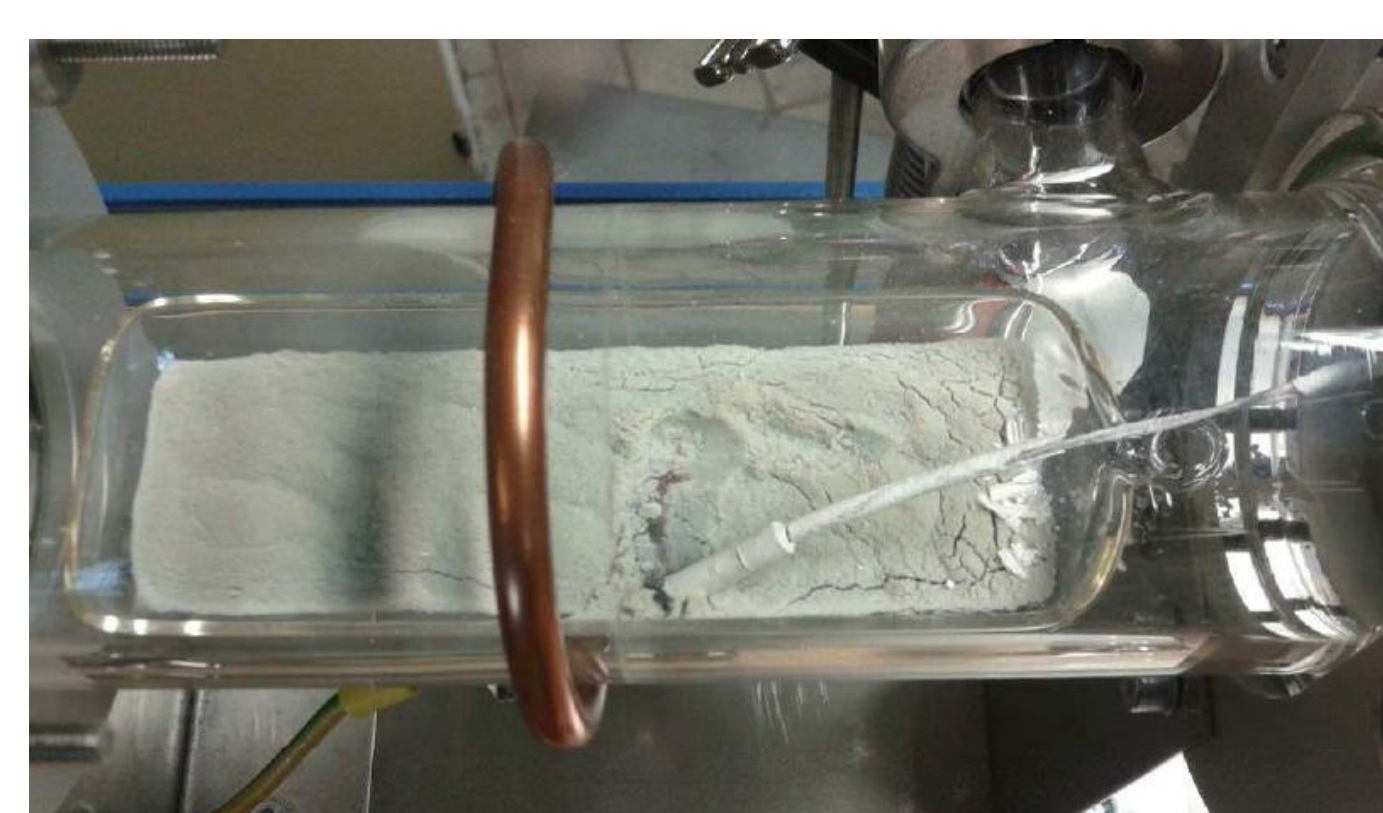
Fig. 2: Result of initial very low temperature ashing experiment for coke sample
