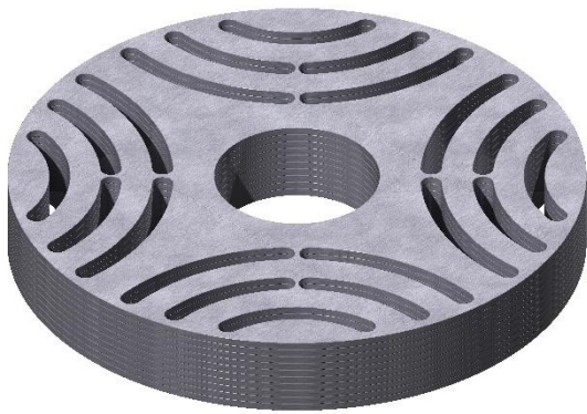
Figure 1: Schematic rotor construction of typical SynRM.
