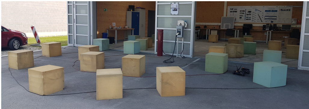
Figure 5.4: Picture of the course setup for the experimental user study. Foam cubes are used as obstacles. Around these, cables are used to mark the bounds of the course.
