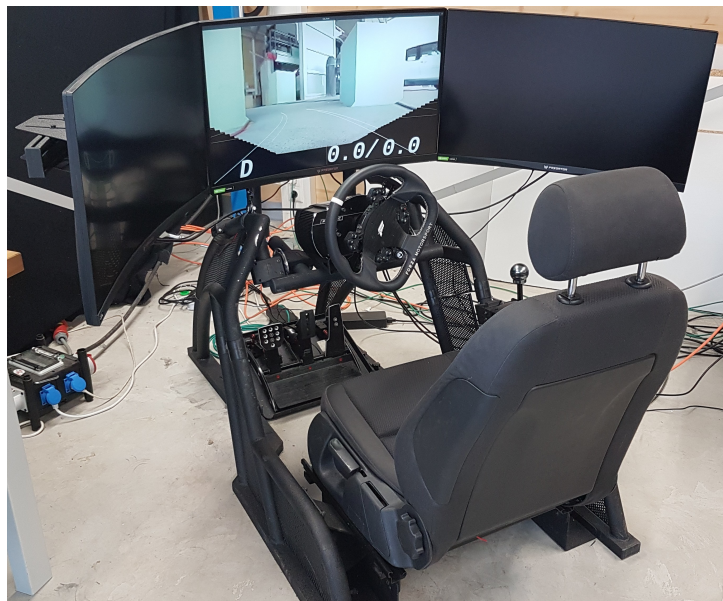
Figure 5.3: Picture of the remote operator desk used in the experimental user study. It is equipped with a Fanatec gaming wheel and pedals, three monitors mounted in a circular shape and a seat.
