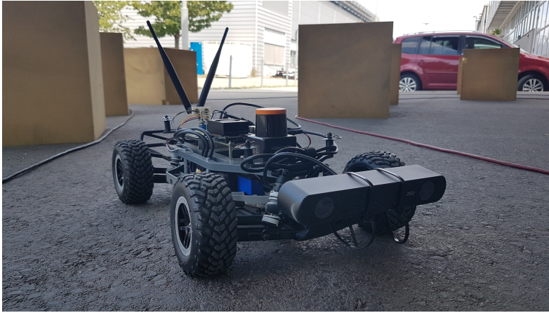
Figure 5.2: Picture of the 1:10-scale vehicle testbed teleoperated in the experimental user study. On board, it is equipped with a 2D LiDAR sensor, a stereo camera, and an NVIDIA Jetson Xavier NX with six cores.
