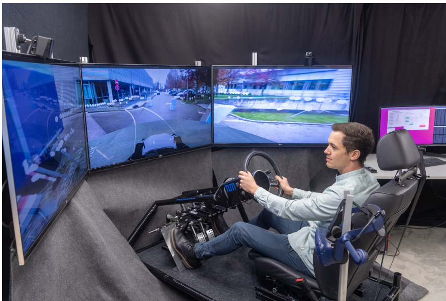
Figure 1.1: Picture of a remote operator performing remote driving. The remote workstation consists of three monitors for the visualization of data from the vehicle. Commands for the vehicle are created using a steering wheel and pedals.
