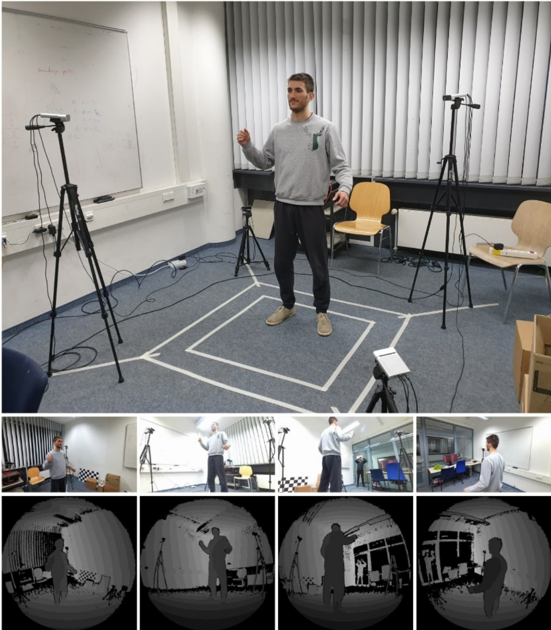
Figure 5.6: Capture setup. We capture non-rigid motion using 4 Kinect Azure sensors, which are pre-calibrated and hardware-synced to guarantee spatial and temporal coherence of depth captures. We capture depth images at resolution of 1024 \times 1024 , using the highest available frame-rate of 15 FPS.
