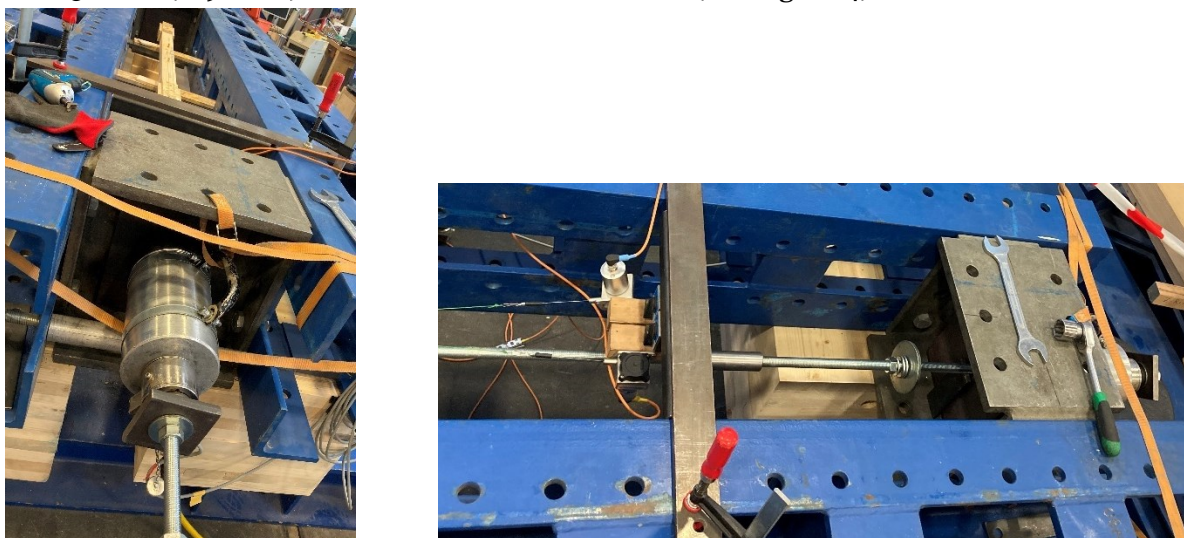
Figure 4: Load application (left) and connection to specimen (right) in the steel frame
