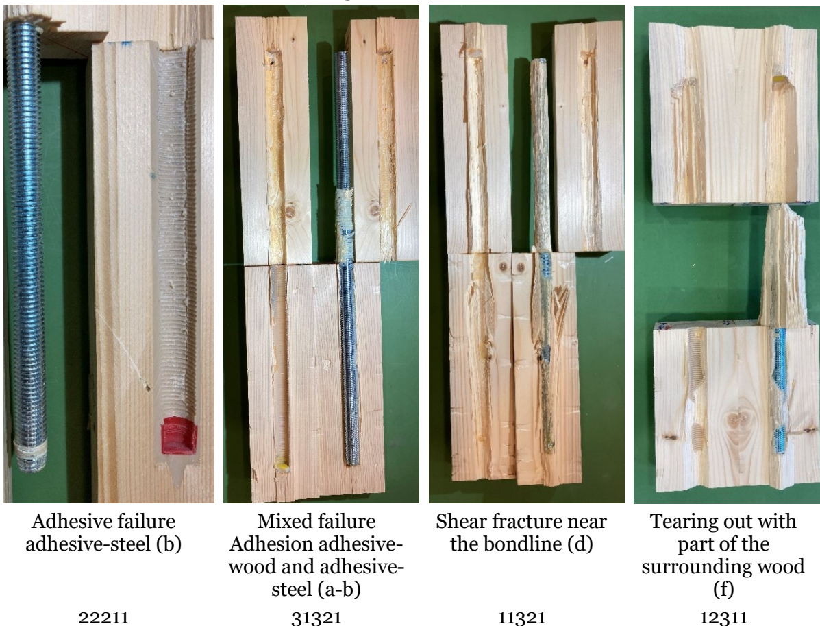
Figure 11: Common failure modes in test series 3
