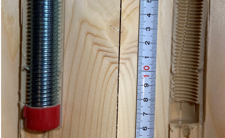
Figure 2: Spacer for the centering of the rod with a glue line thickness of 3 mm
