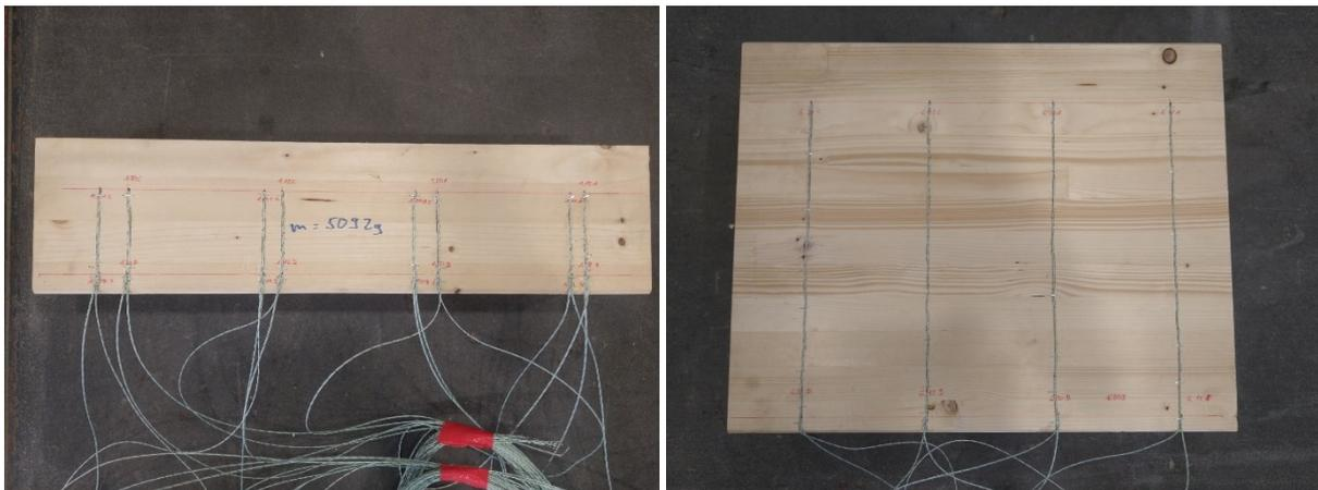
**Figure 10: Routing of thermocouples on the edges of the specimens**
