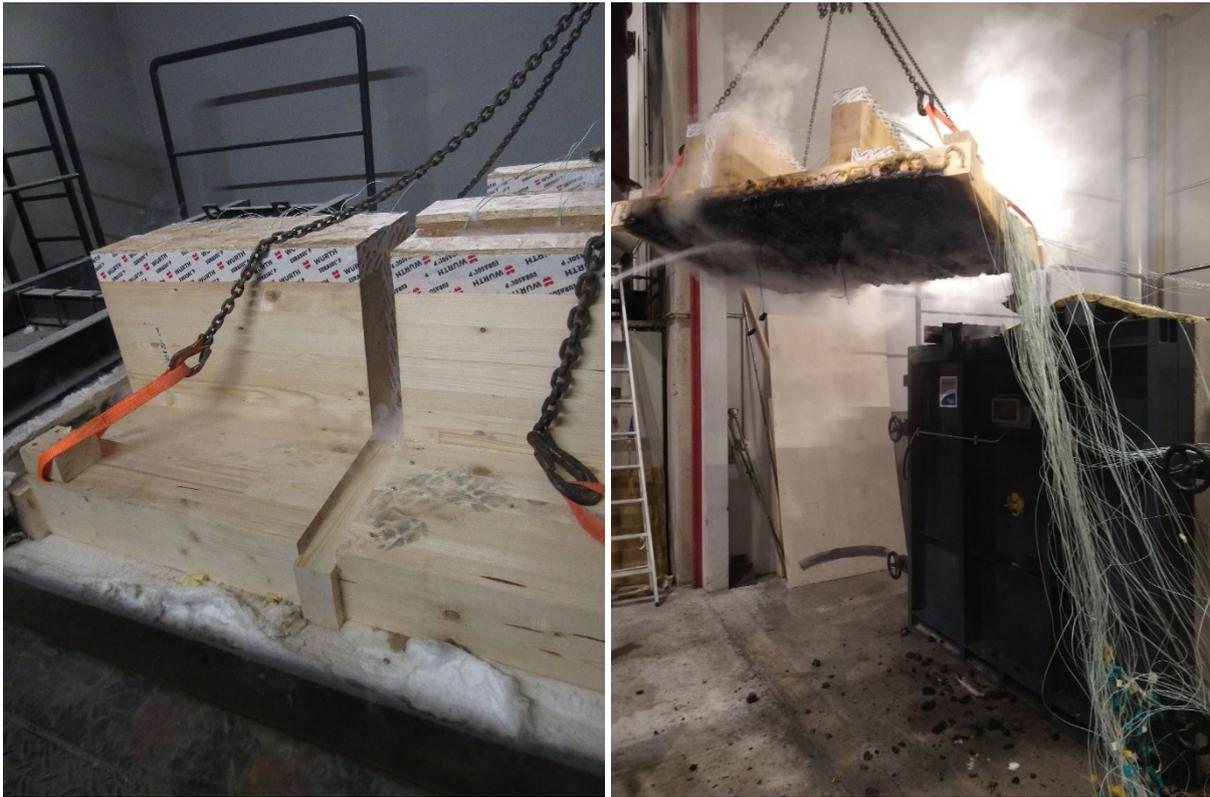
**Figure 20: left: Specimen during the fire test with slight plumes of smoke; right: Lifting of the ceiling after the fire test**
