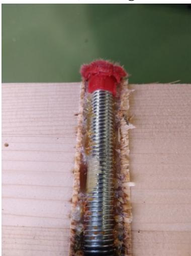
**Figure 32: Melting of plastic cap on the unexposed surface**
