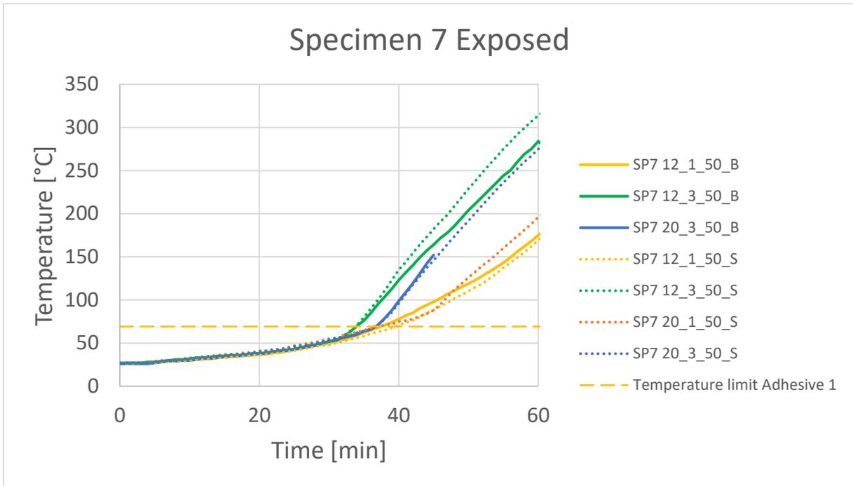
**Figure 34: Measured temperatures of Specimen 7 on the exposed surface**
