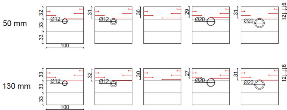
**Figure 2: Planned and built location of the thermocouples in test series 2.1**
