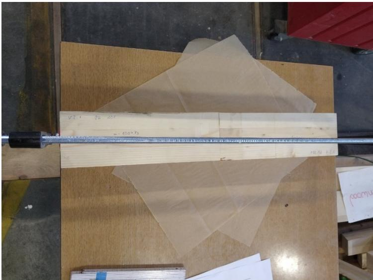
**Figure 4: Gluing process for specimen 121**
