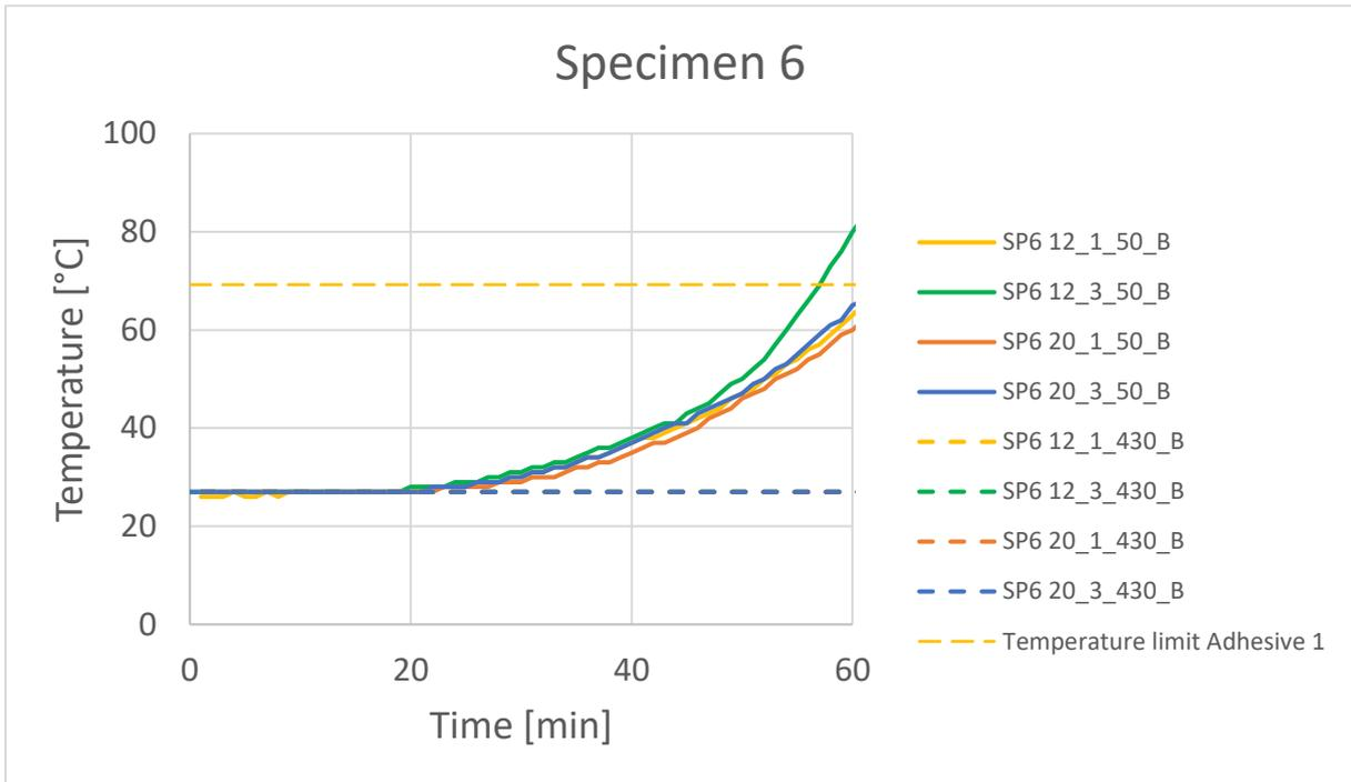
**Figure 59: Temperature curves for specimen 6 of test series 2.2**
