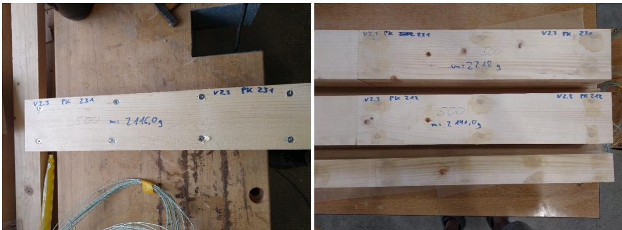
**Figure 14: left: Screwing together of the two specimen halves, right: Sealing of the screw holes**
