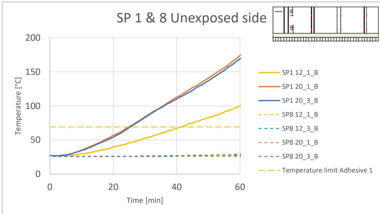
**Figure 37: Measured temperatures of Specimens 1&8 on the unexposed surface**
