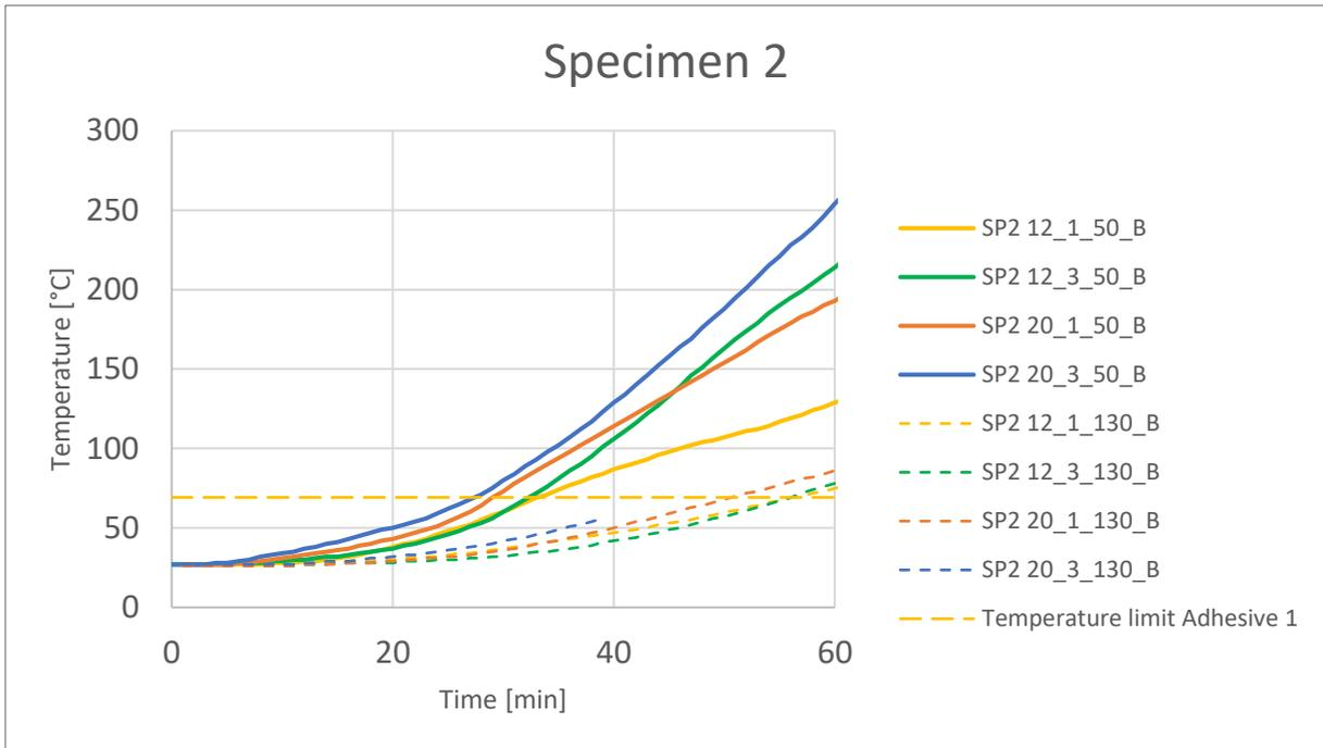
**Figure 55: Temperature curves for specimen 2 of test series 2.2**
