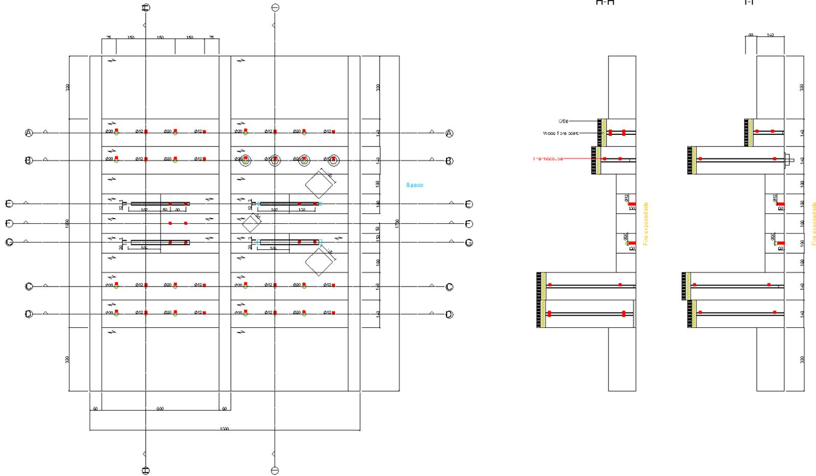
Figure 47: Top view and sections of test specimen in test series 2 (red: thermocouples)
