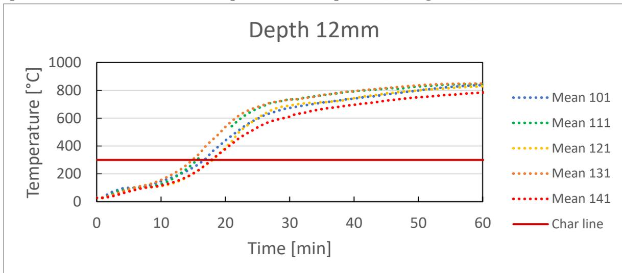
**Figure 25: Measured temperature for a depth of 12 mm from the fire exposed side**
