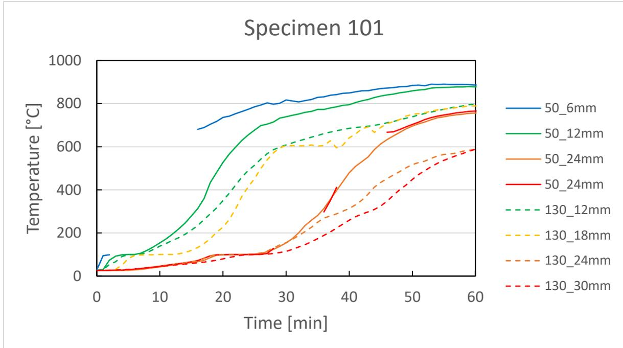
Figure 48: Temperature development in specimen 101 for the measurement positions in a distance of 50 mm and 130 mm of the joint
