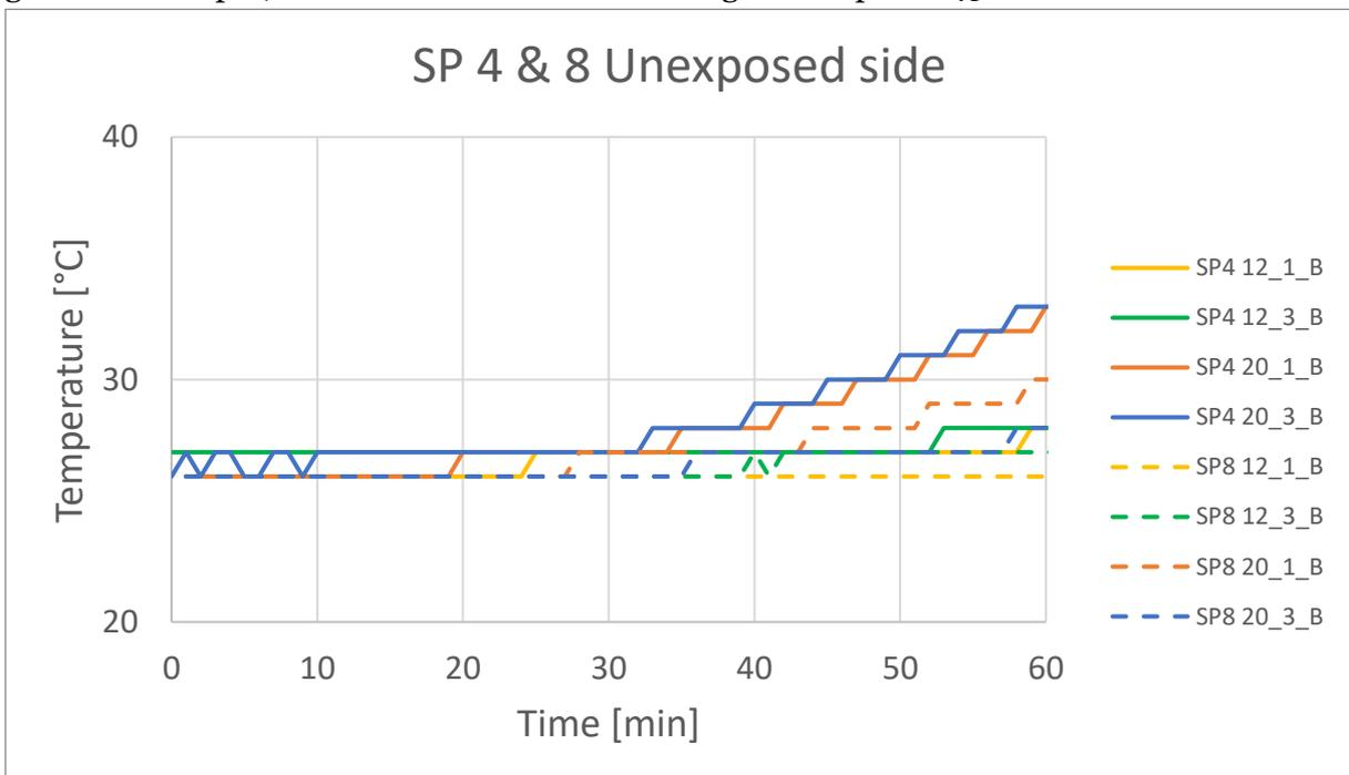
**Figure 43: Measured temperatures of Specimens 4&8 on the unexposed surface**
