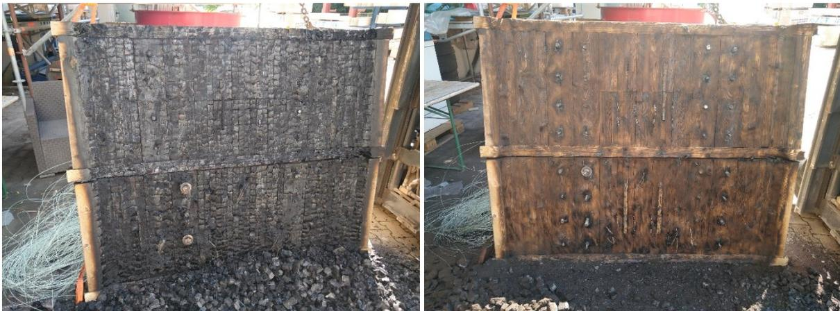
**Figure 21: View of fire exposed side after cooling on the left and after cleaning of the charcoal layer on the right**
