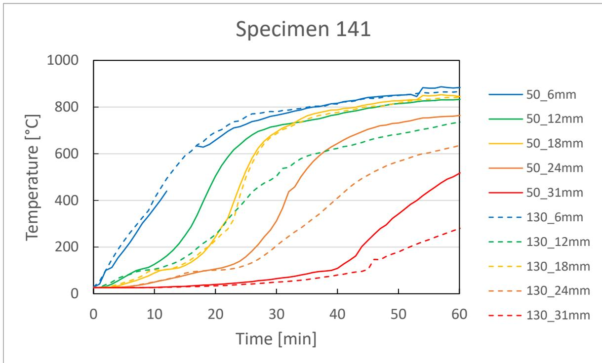
Figure 52: Temperature development in specimen 141 for the measurement positions in a distance of 50 mm and 130 mm of the joint
