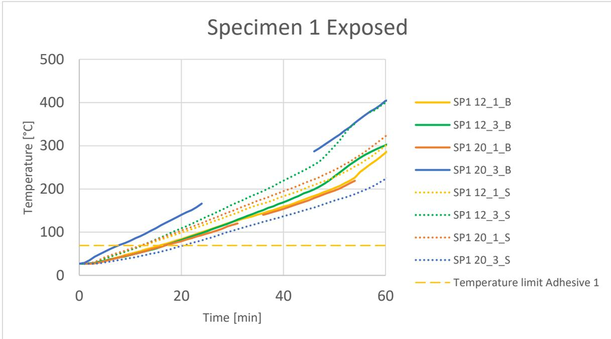
Figure 53: Temperature curves for specimen 1 of test series 2.2 on the side exposed to fire
