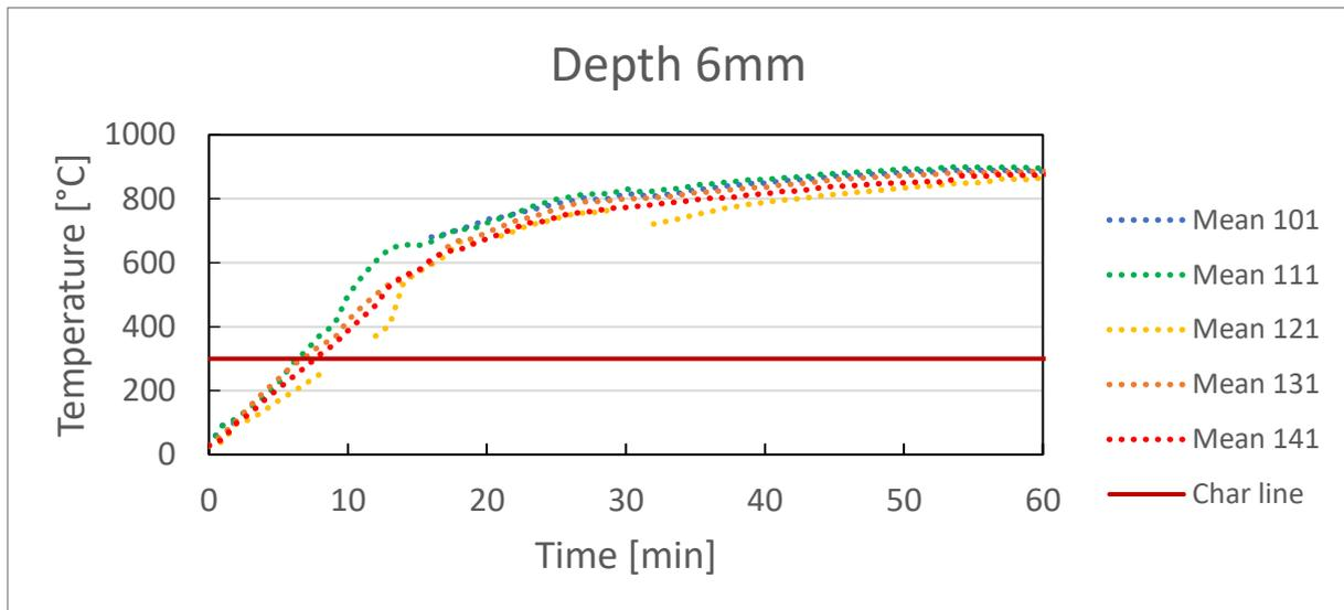
**Figure 24: Measured temperature for a depth of 6 mm from the fire exposed side**
