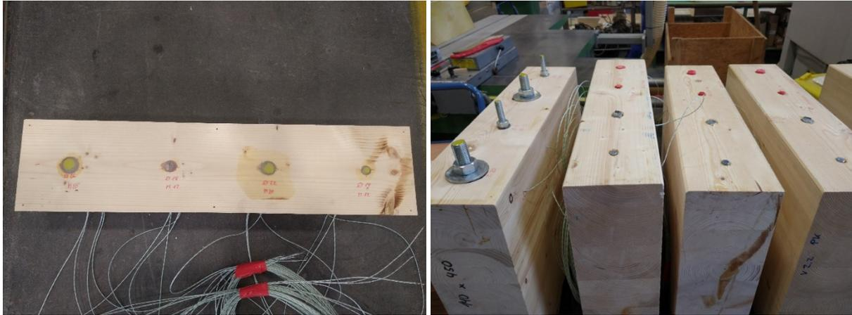
**Figure 9: Surfaces of the specimens after gluing and removal of the oriented strand board**
