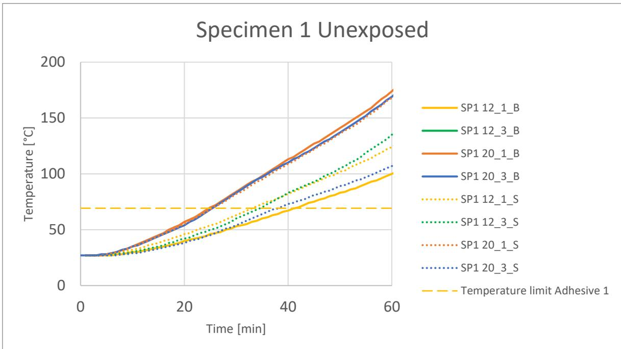
Figure 54: Temperature curves for specimen 1 of test series 2.2 on the side unexposed to fire
