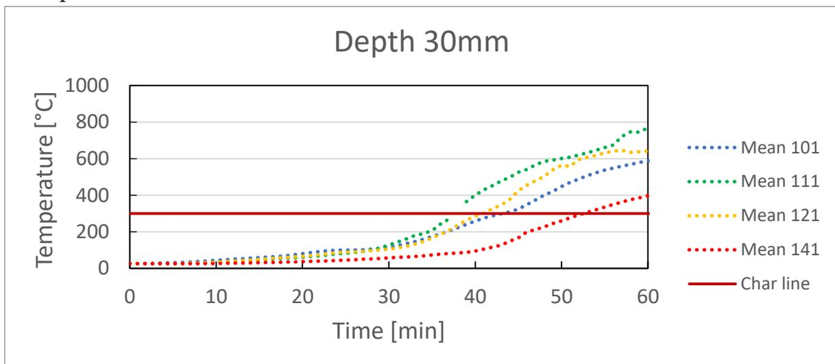
**Figure 28: Measured temperature for a depth of 30 mm from the fire exposed side**
