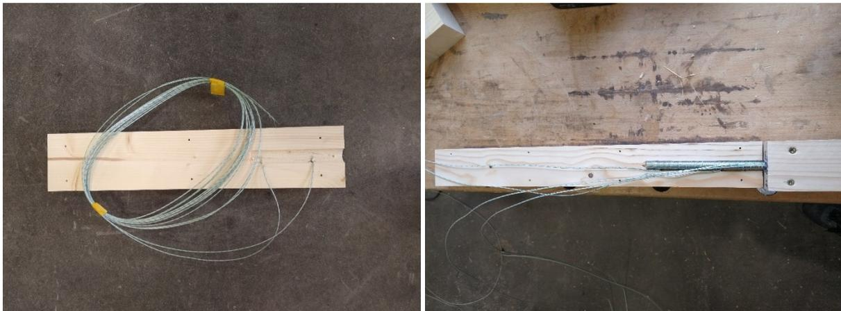
**Figure 13: Inserting of the thermocouples**
