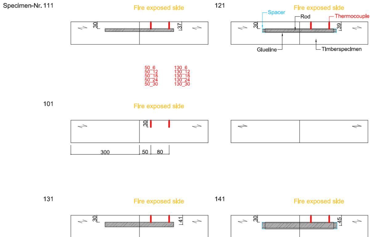
**Figure 1: Sketch Specimens in test series 2.1 (red: thermocouples, blue: spacer)**
