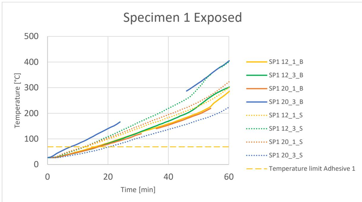
**Figure 31: Measured temperatures of Specimen 1 on the fire exposed surface**
