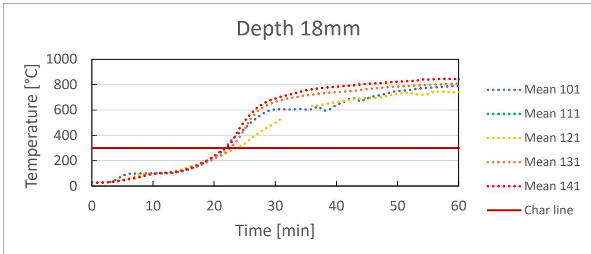
**Figure 26: Measured temperature for a depth of 18 mm from the fire exposed side**
