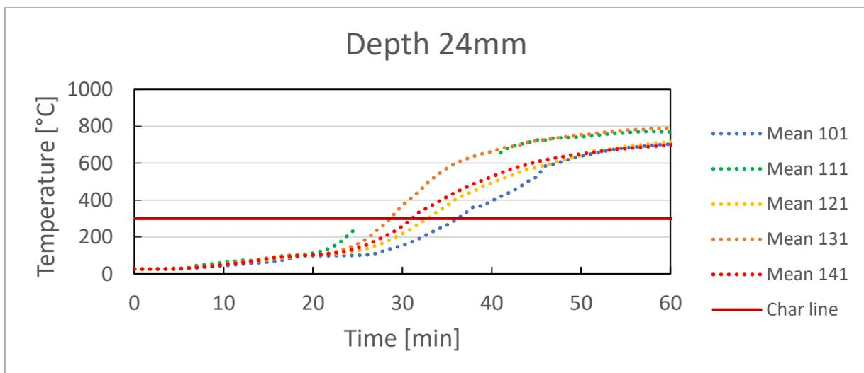
**Figure 27: Measured temperature for a depth of 24 mm from the fire exposed side**
