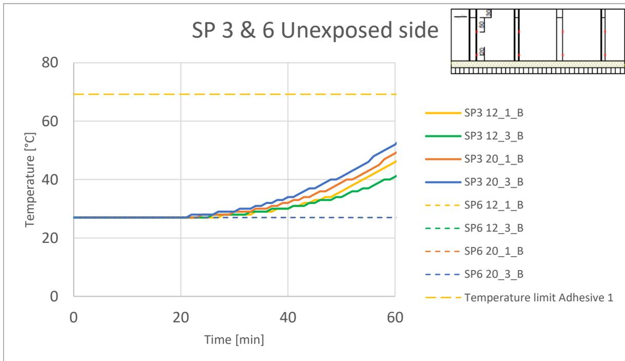
**Figure 41: Measured temperatures of Specimens 3&6 on the unexposed surface**
