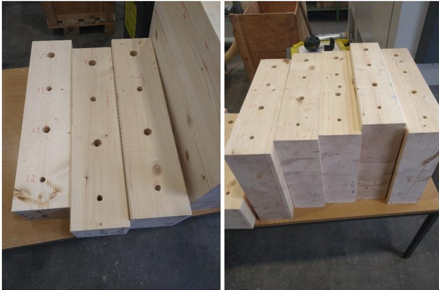
**Figure 6: Drilled specimens 1 -3 on the left and 4 – 8 on the right**
