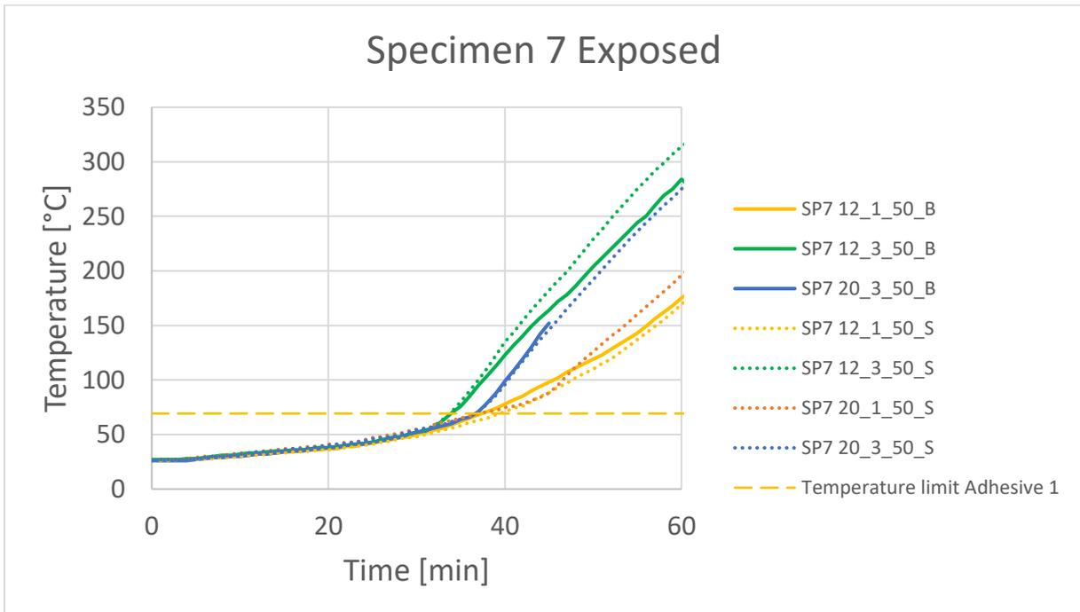
**Figure 60: Temperature curves for specimen 7 of test series 2.2 on the side exposed to fire**
