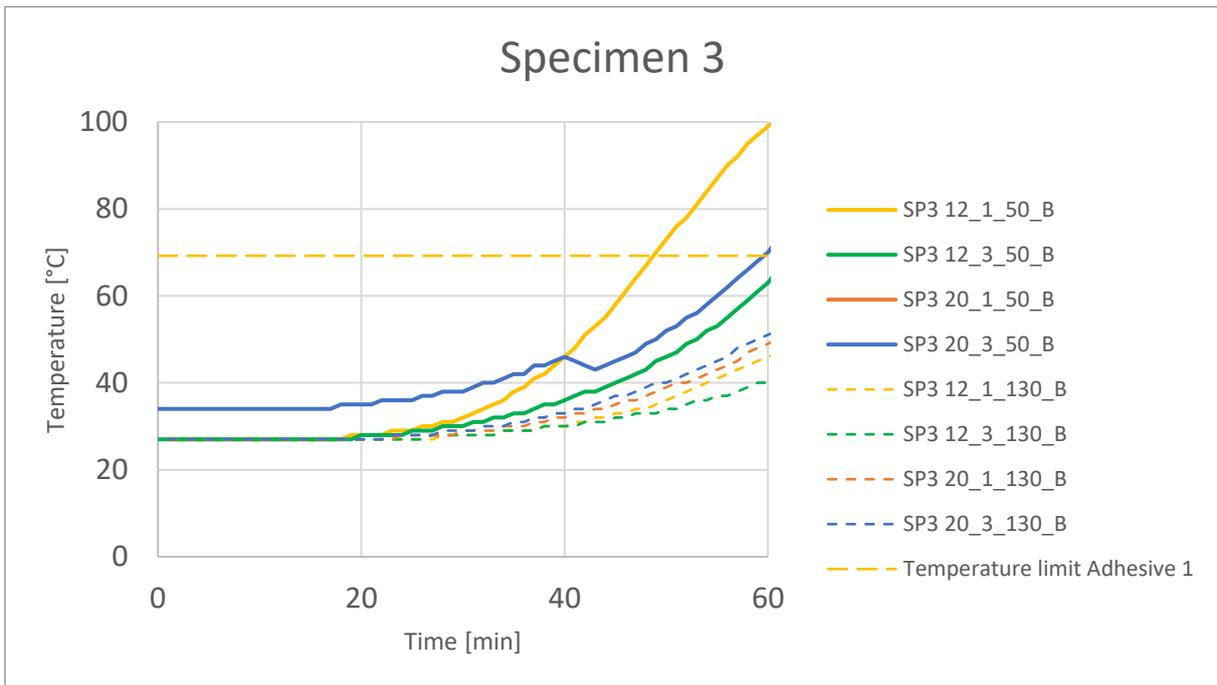
**Figure 56: Temperature curves for specimen 3 of test series 2.2**
