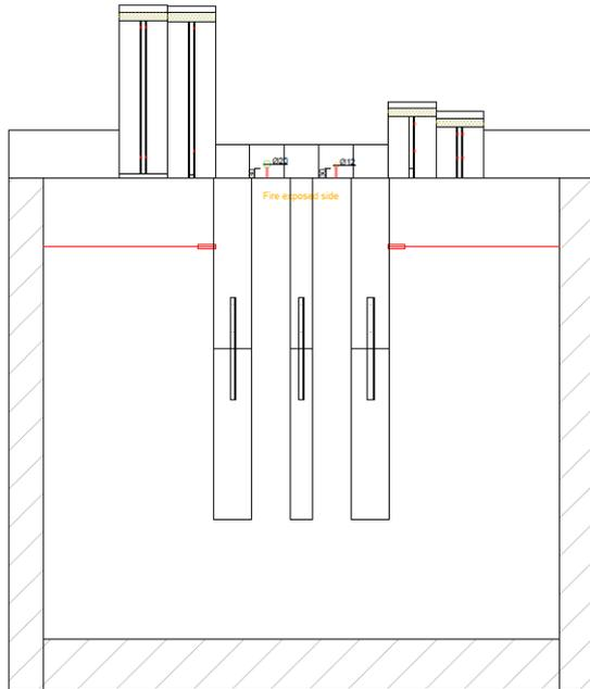
**Figure 18: View of the furnace with built-in specimen and thermo plates (red)**
