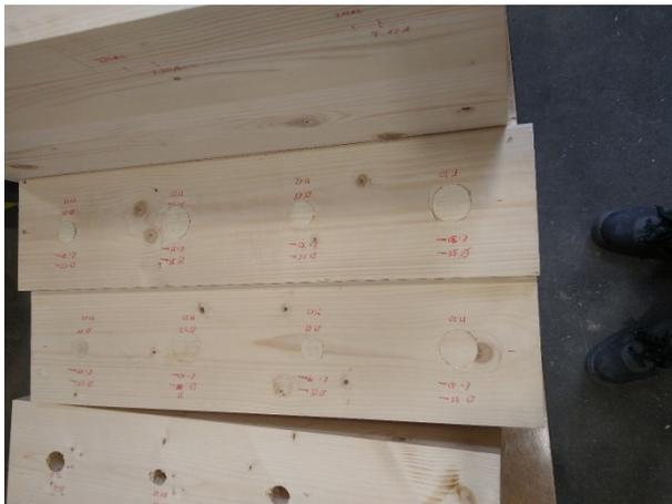
**Figure 7: Specimens with inserted wooden plugs**
