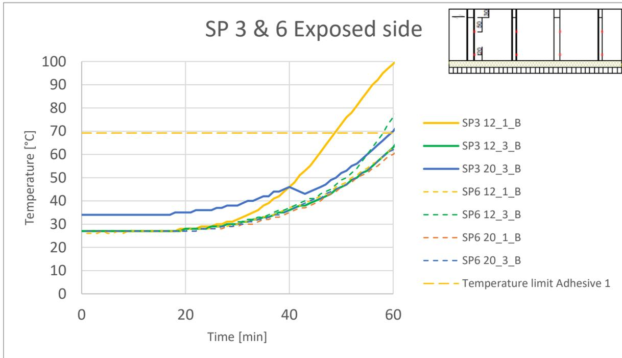
**Figure 40: Measured temperatures of Specimens 3&6 on the fire exposed surface**
