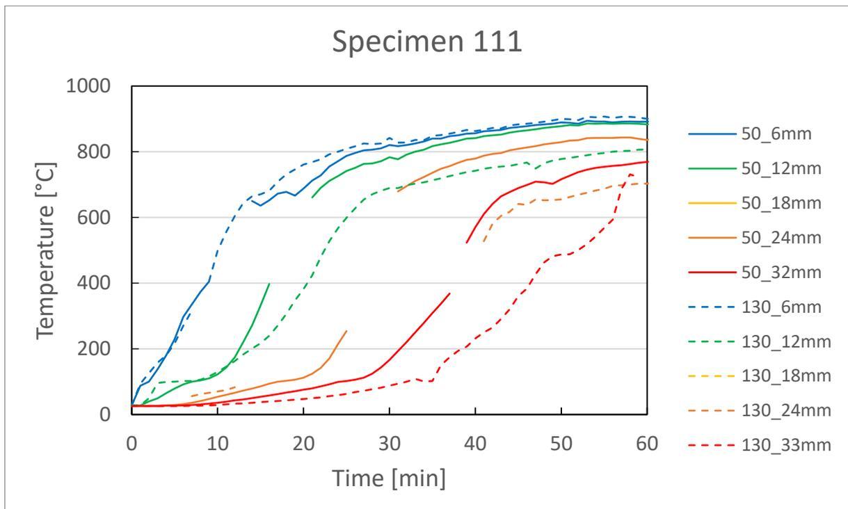
Figure 49: Temperature development in specimen 111 for the measurement positions in a distance of 50 mm and 130 mm of the joint
