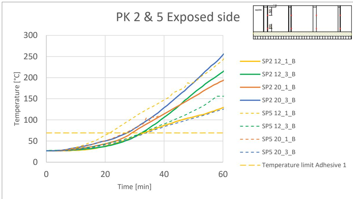
**Figure 38: Measured temperatures of Specimens 2&5 on the fire exposed surface**
