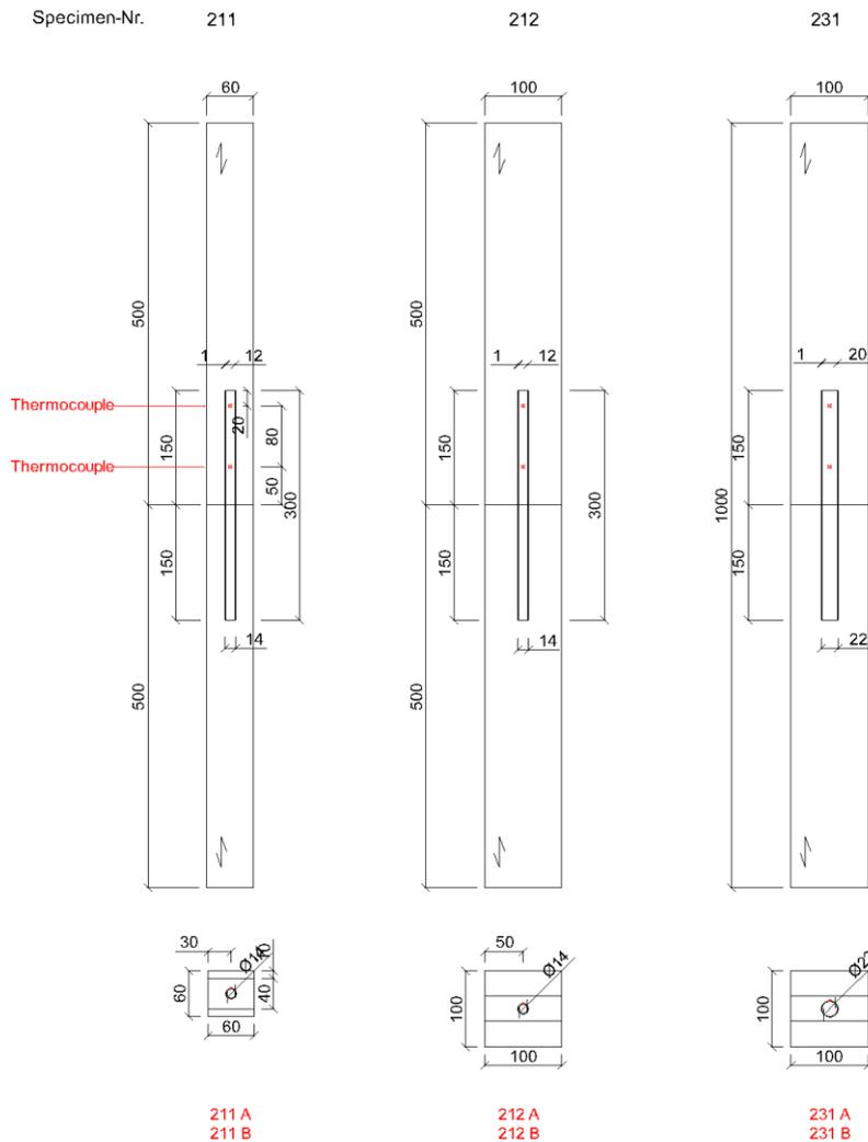
**Figure 12: Dimensions of the specimens in test series 2.3 (red: thermocouples)**
