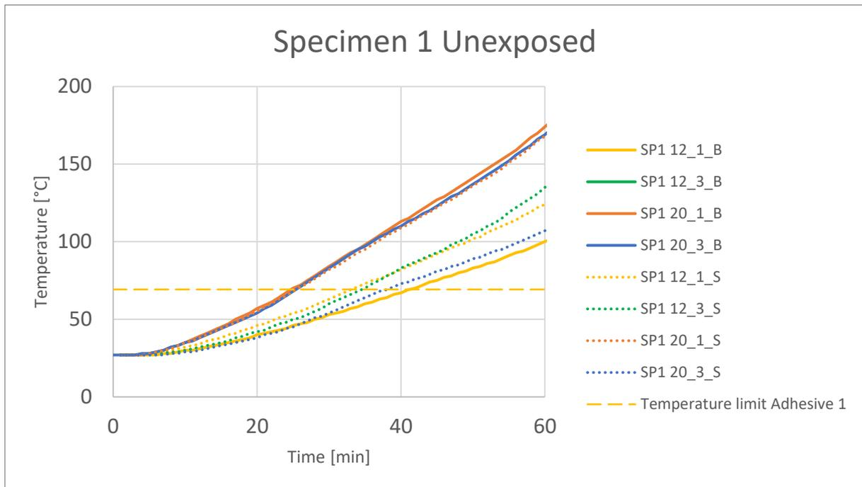
**Figure 33: Measured temperatures of Specimen 1 on the unexposed surface**
