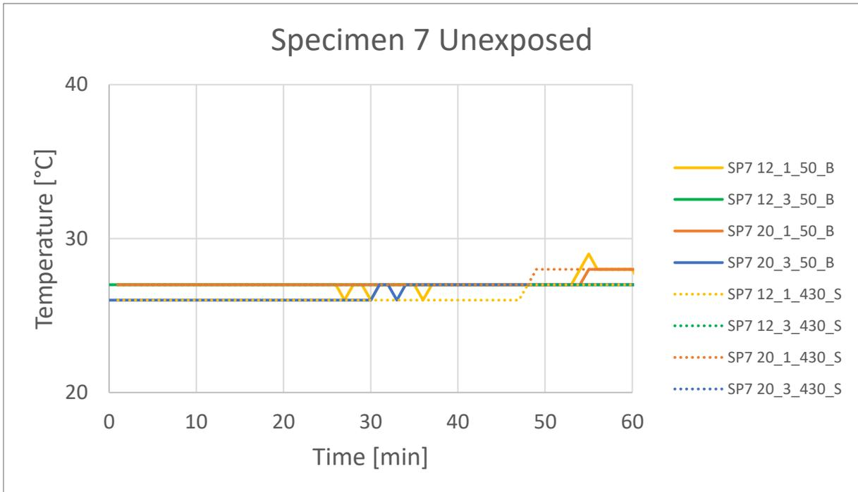
Figure 61: Temperature curves for specimen 7 of test series 2.2 on the side unexposed to fire
