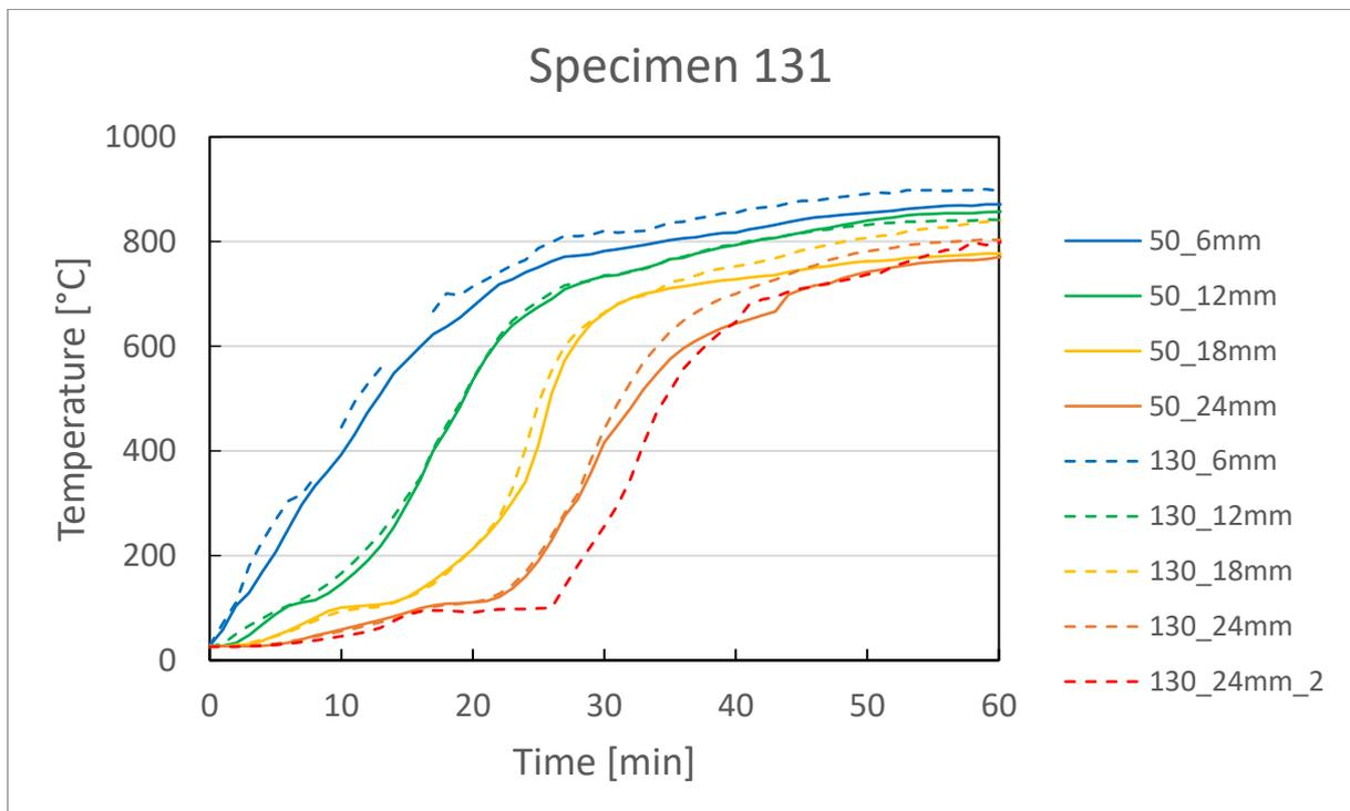
**Figure 51: Temperature development in specimen 131 for the measurement positions in a distance of 50 mm and 130 mm of the joint**
