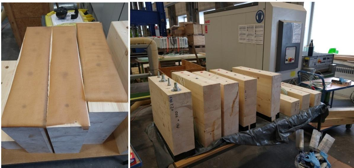
**Figure 8: Specimens before (left side) and during (right side) the gluing process**
