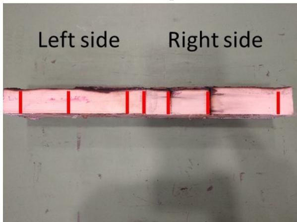
**Figure 22: Measurement points of char depth (red)**
