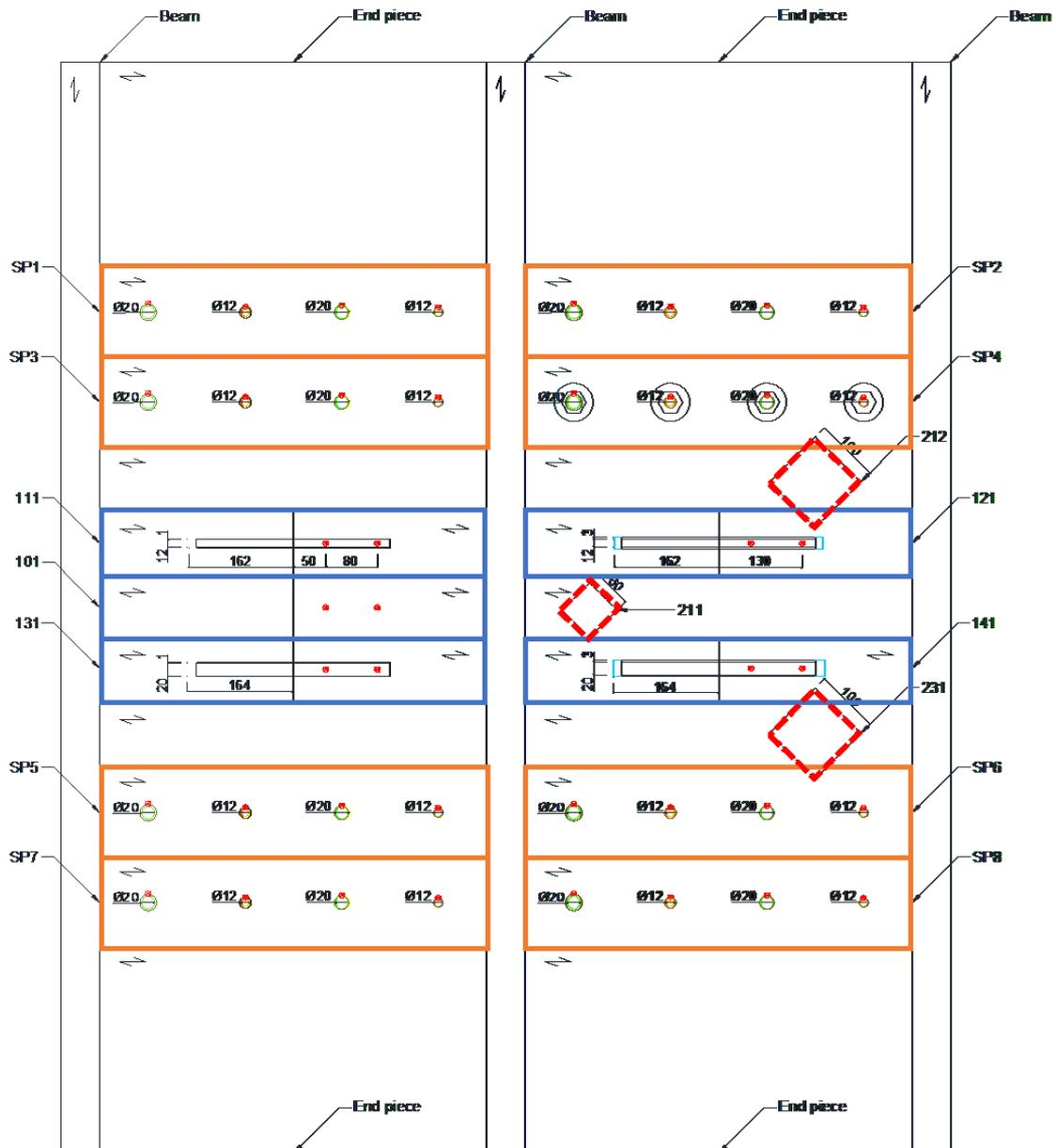
**Figure 15: Sketch of the ceiling specimen for test series 2.1 (blue), test series 2.2 (orange) and test series 2.3 (red)**
