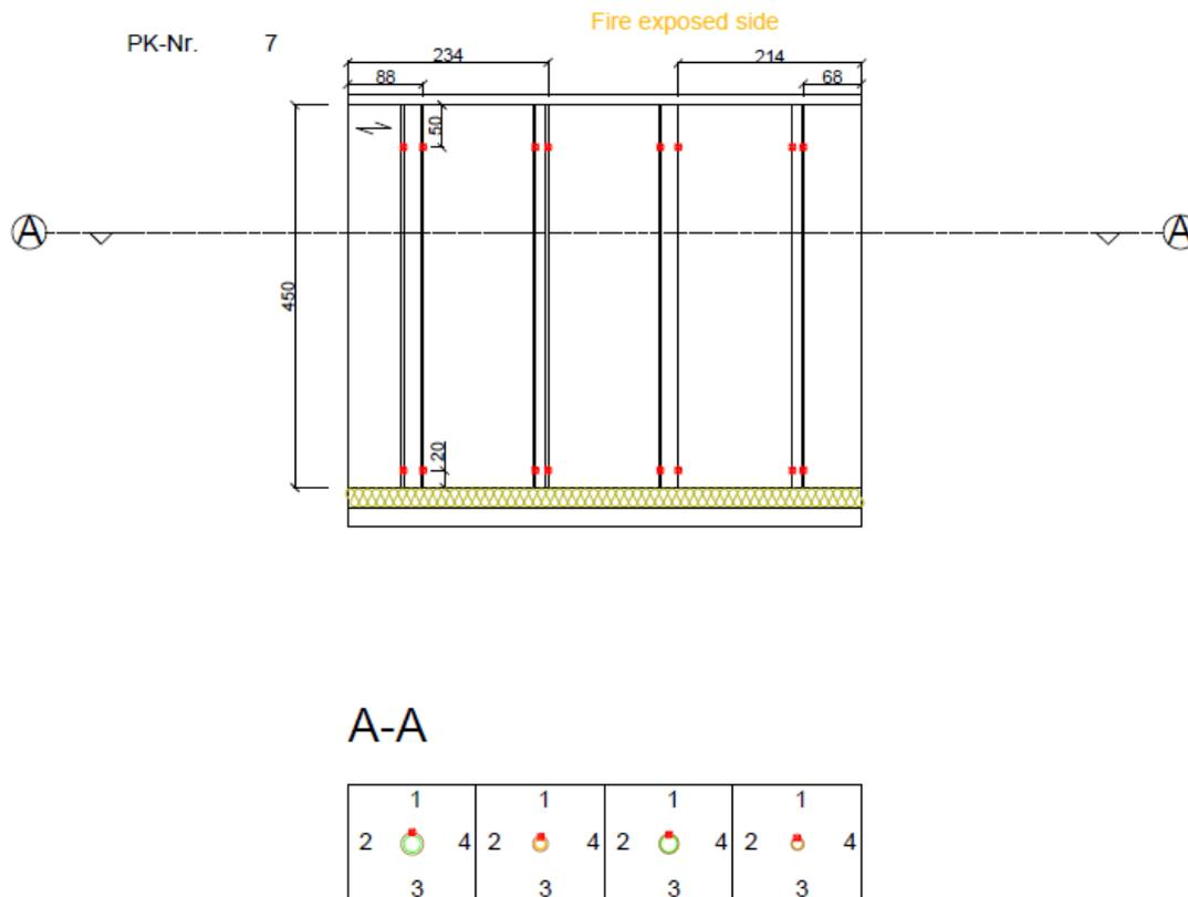
**Figure 29: View of the cutting lines and the numbering of the four sides**
