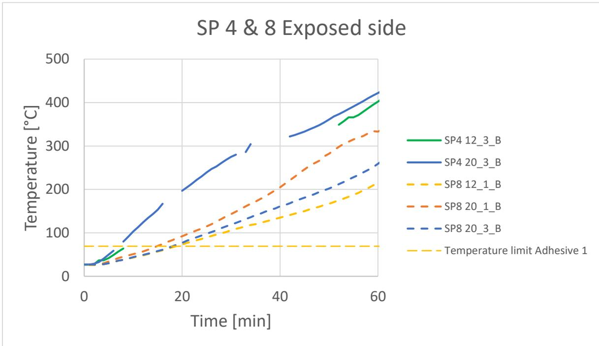
**Figure 42: Measured temperatures of Specimens 4&8 on the fire exposed surface**
