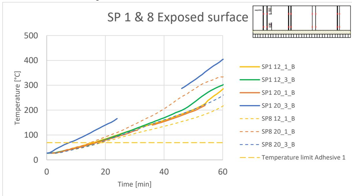
**Figure 36: Measured temperatures of Specimens 1&8 on the fire exposed surface**
