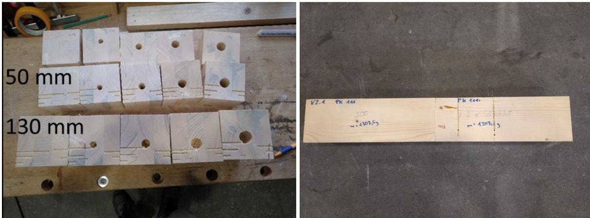
**Figure 3: left: View of the specimens after milling, right: Channels on the side of the specimen**
