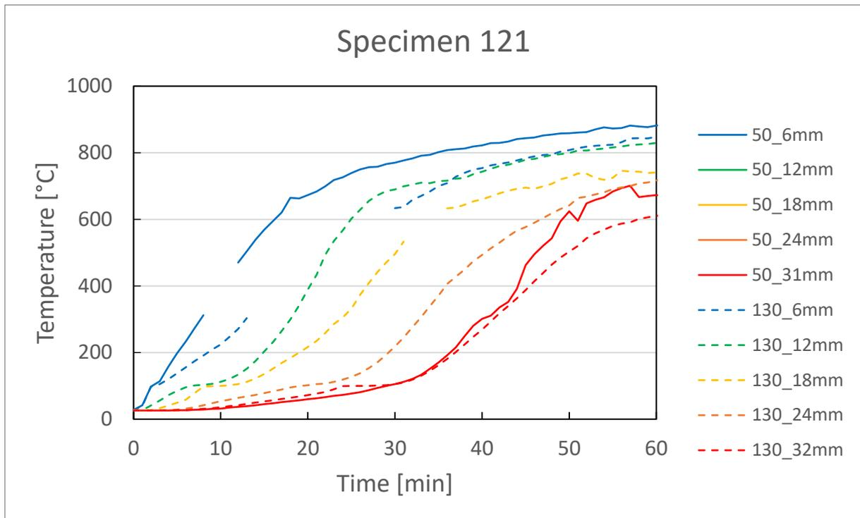
**Figure 50: Temperature development in specimen 121 for the measurement positions in a distance of 50 mm and 130 mm of the joint**
