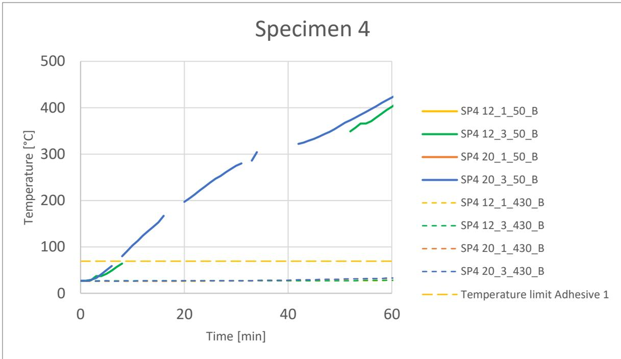
**Figure 57: Temperature curves for specimen 4 of test series 2.2**
