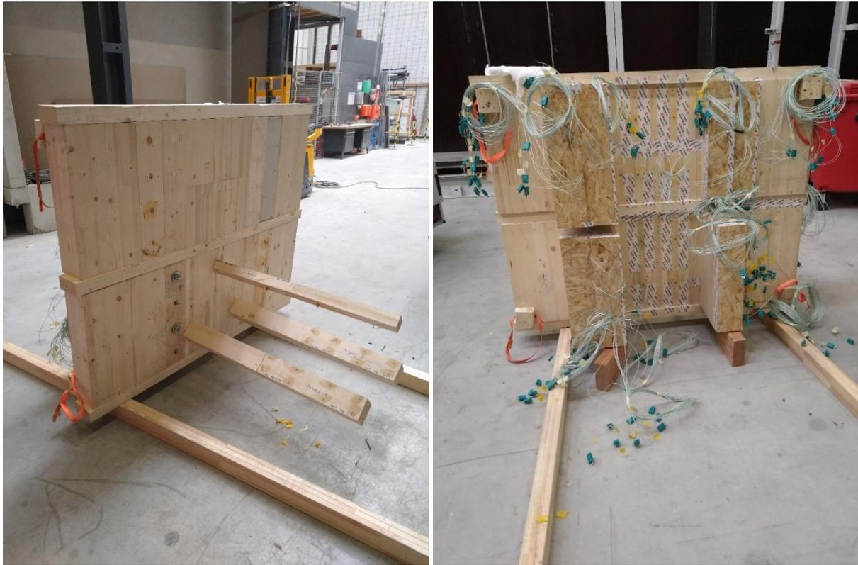
**Figure 17: Finished specimen before the fire test (left: side exposed to the fire, right: unexposed side)**
