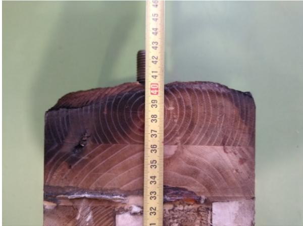
**Figure 30: View of side 2 of specimen 6 with higher charring on the edges**
