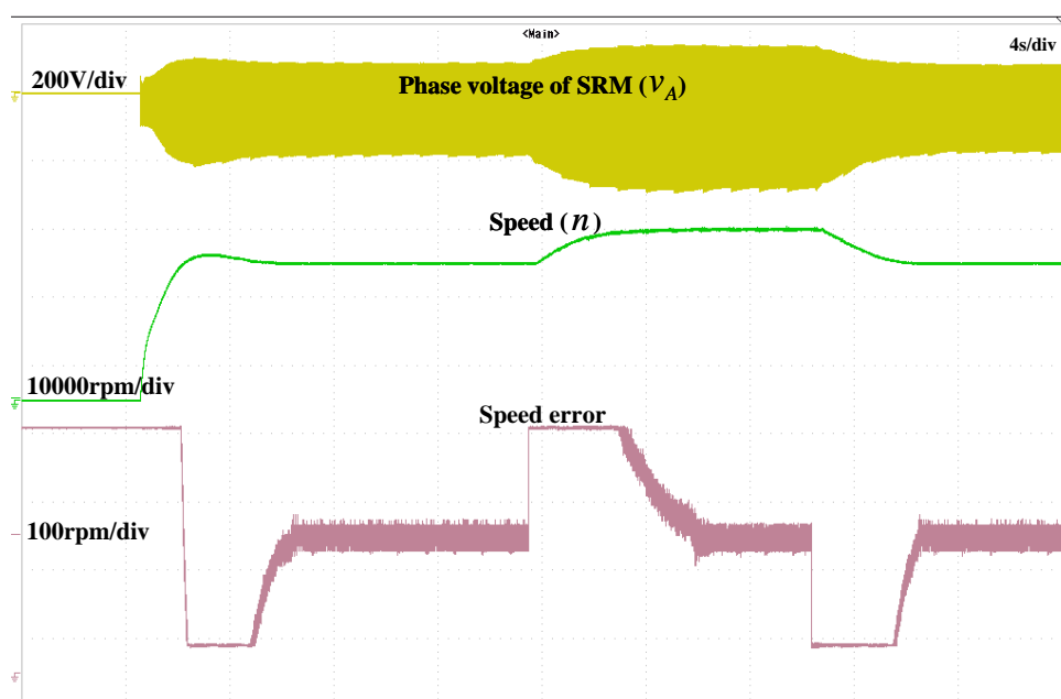
Figure 3.20: Dynamic test results when speed changes from 0 r/min to 20000 r/min to 25000 r/min to 20000 r/min.
