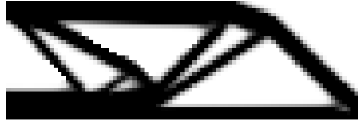
Figure 6.4: The optimized MBB beam using the conventional SIMP method with 90 \times 30 density elements and a filter radius of r_{min} = 1.5 .
