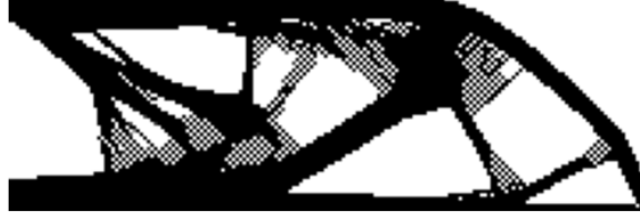
Figure 3.2: The optimized MBB beam solved with bilinear quadrilaterals and without any regularization method. Checkerboard patterns occur in the final design.
