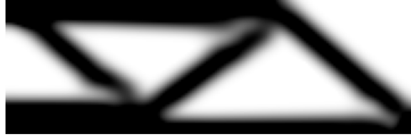
Figure 4.3: The optimized MBB beam solved with bilinear quadrilaterals and the multi-resolution scheme. Sensitivity filtering with a radius of r_{min} = 7h_v is applied.
