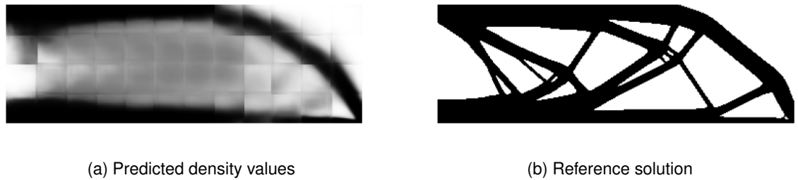
Figure 6.13: Prediction of the density field based on the initial stress and strain terms. The individual subdomains are joined after the NN prediction.
