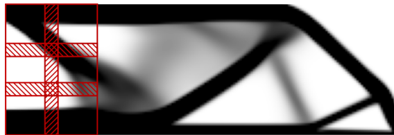
Figure 5.7: Overlapping areas occur if the design space can not be decomposed exactly into subdomains of size 32 \times 32 .
