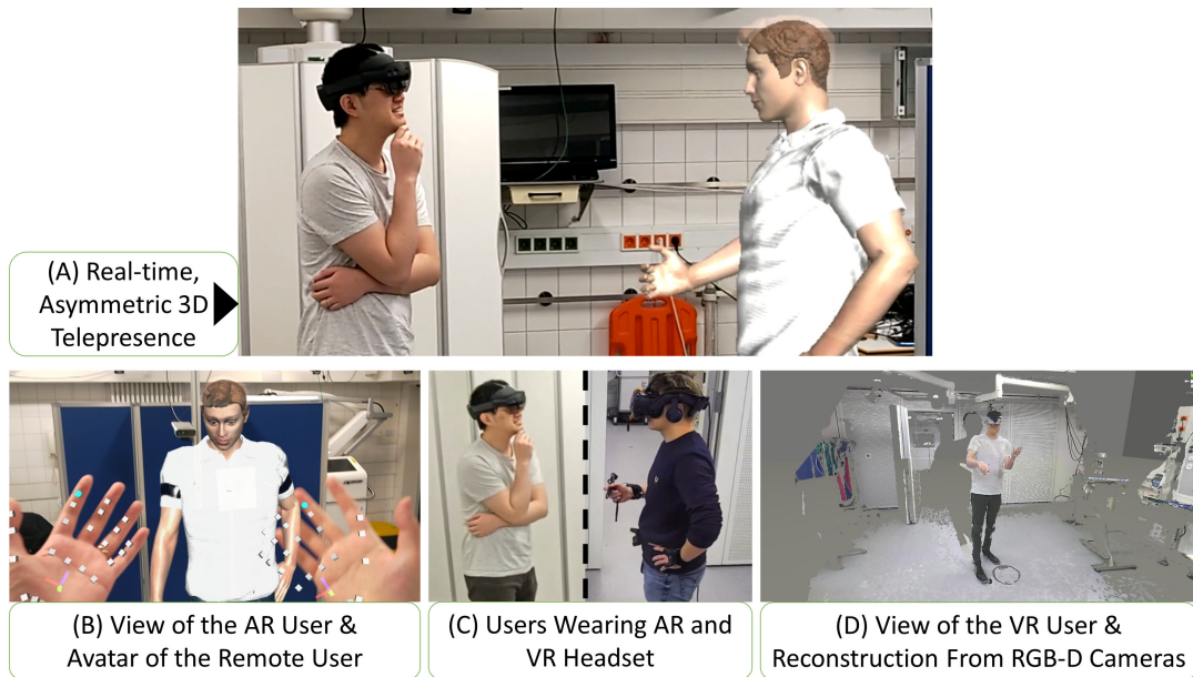
Fig. 1.4. 3D Telepresence using Augmented and Virtual Reality. (A) Local users wearing an AR headset (here Hololens 2) see the remote-connected VR user. Both users can see the surrounding environment of the local user. (B) The AR user can communicate with the VR user in a face-to-face manner. (C) Both users are physically separated; However, telepresence connects both as if they would share a common space. (D) The feeling of being there is created by capturing the local environment with RGB-D camera and re-project the data into a 3D reconstruction.
