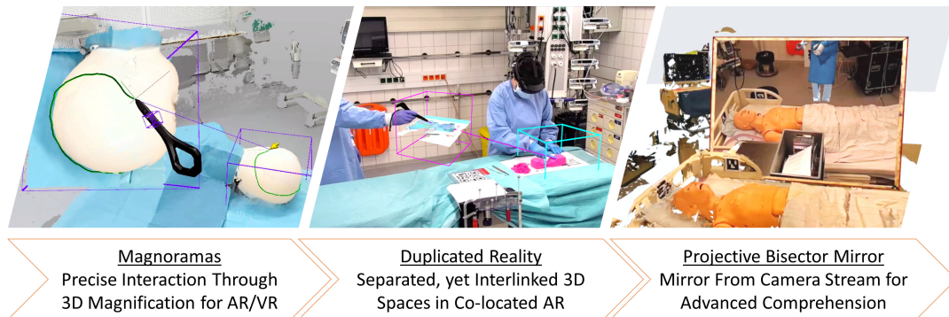
Fig. 1.2. This Dissertation’s Three Interaction Methods to Enhance Medical Consultation. The Magnorama enhances dynamic interactions with the 3D environment, particularly for creating mid-air annotations. The Duplicated Reality is the continuation of Magnoramas and investigates its ability to utilize 3D space more efficiently and maintain task performance. Finally, the Projective Bisector Mirror provides additional high-fidelity views from the scene reconstructed from RGB-D cameras to enhance the comprehension of the virtual scene.
