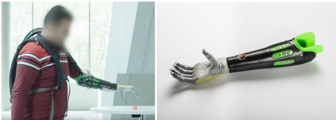
**Fig. 1** Prosthetic setup in our study; On the left: Participant P wearing custom-build hardware consisting of a small backpack housing hardware for data acquisition and wireless communication and a battery. On the right: Custom-built socket with eight snap-on electrodes uniformly distributed around the circumference of the stump. The prosthetic hand was the i-LIMB Revolution (Össur hf)
