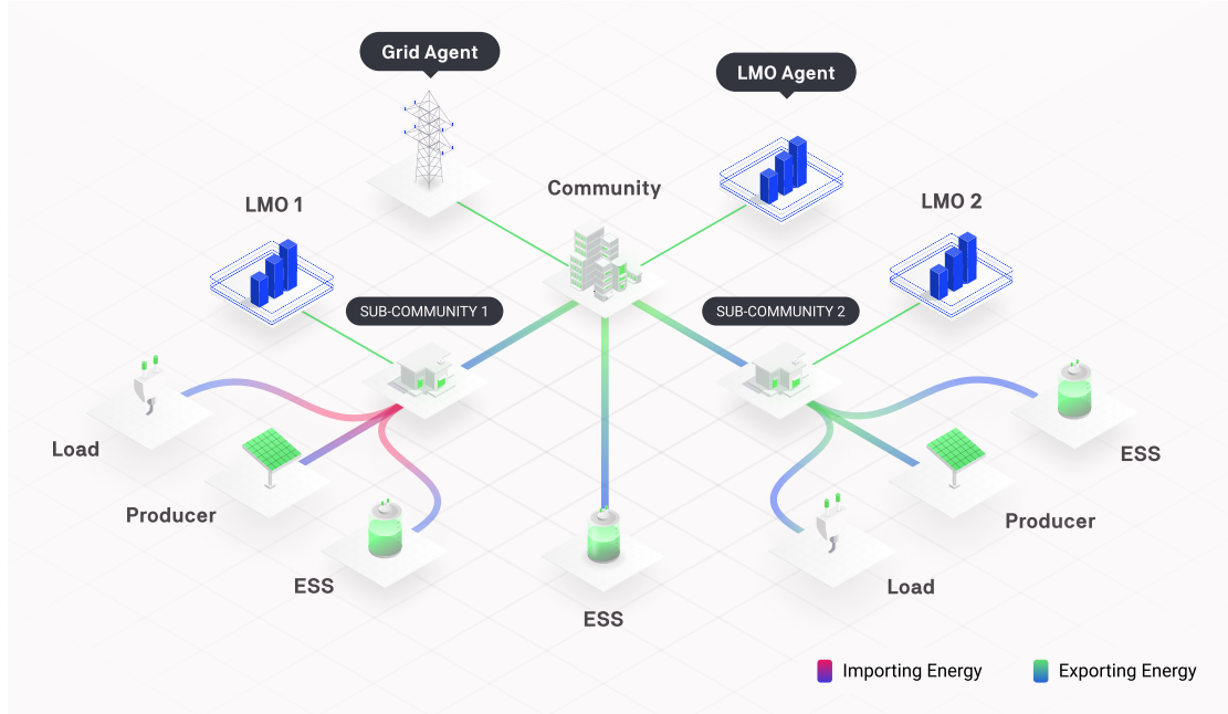
Figure 3.1: Schematic of hierarchical multi-agent model developed using Grid Singularity exchange [120]. Figure adopted from [130].
