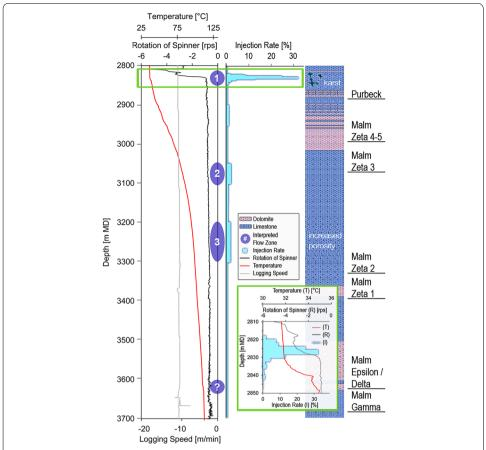
**Fig. 6** Interpreted flow zones in producer well together with flowmeter spinner data, temperature and logging speed, lithology and stratigraphic units. Zoom to top section is shown in green framed box
