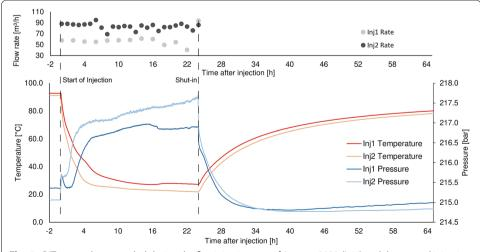
**Fig. 4** *P/T* gauge data recorded during the first injection test of January 2020 (Inj1) and the second injection test of February 2020 (Inj2) with injection rates
