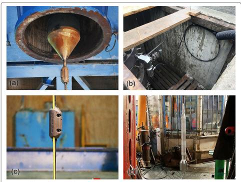
**Fig. 2** Installation of the FO-cable in the producer well. **a** ¾-in. to 13 3/8-in. crossover. **b** Wellhead outlet. **c** TEF mounted on sucker rods with clamps. **d** Carrier at termination with centralizer
