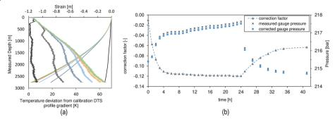
**Fig. 13** Calculated strain from DTS and corrected pressure data. **a** Calculated strain from DTS data to the depth of the *P/T* gauge in the first 7 h of injection of Inj2. Curves on the left y-axis are temperature deviations from the initial DTS profile. Curves on the right y-axis are the resulting strain for each DTS profile. **b** Measured gauge pressure data with correction factor to revise thermal caused displacement
