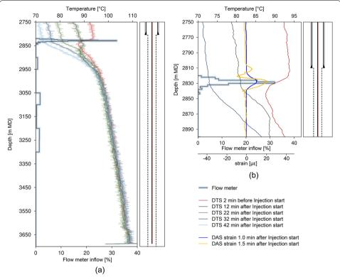
**Fig. 14** Comparison of flowmeter injection profile and DTS and DAS response during Inj2. Transparent lines are raw DTS data, sharp lines are moving average over 10 m. **a** Flowmeter profile with five DTS profiles in the first hour of cold water injection over from 2750 m MD to TD. **b** Zoomed to top of the reservoir. Flowmeter profile is shown together with three DTS profiles of injection start, each 20 min apart; and DAS strain at 1 min and 1.5 min after injection start
