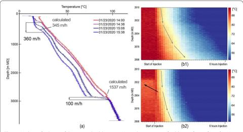
**Fig. 9** Analysis of velocity of the injected cold water. **a** Vertical movement of cold waterfront of Inj1. **b1** Heat plot of Inj1. **b2** Heat plot of Inj2. Gray arrows: suggested 75 °C isotherm. The black arrow marks the proposed major hydraulic active zone
