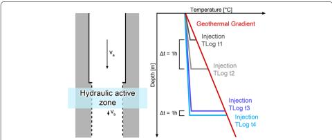
**Fig. 5** Schematic DTS velocity track analysis during injection of cold water. Dark gray and light gray lines are DTS temperature logs (TLog) at different times t1 and t2 and show the downhole propagation of injected cold water in the cased section of a well. Dark blue and light blue lines are DTS profiles at later times t3 and t4 below a feed zone.  $v_a$  and  $v_b$  are the velocities above and below the hydraulic active zone
