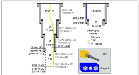
**Fig. 1** Completion of production well 1 (left) and injection well 2 (right) with equipped fiber optic cables in Munich with relevant depths and kick-off points (KOP). Blue: with bumper wires equipped flatpack cemented (gray) behind the casing in injector well. Yellow: tubular encased fiber (TEF) installed along sucker rods to TD in producer well. Turquoise: fiber optic *P/T* gauge. Sketches of TEF and Flatpack are shown in gray box
