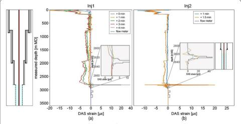
**Fig. 8** DAS strain measurements at the beginning of injection tests Inj1 (a) and Inj2 (b). The gray line marks the injection profile from flowmeter. DAS strain at the top of the reservoir is given in zoomed in sub plots
