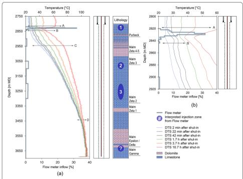
**Fig. 15** Comparison of DTS warm-back profiles and flowmeter injection profile with interpreted injection zones from flowmeter interpretation. Transparent lines are raw DTS data, sharp lines are moving average over 10 m. **a** Six DTS profiles taken at different times during the first 11 h together with flowmeter inflow profile. A, B, C and D mark gradient change of DTS profiles. **b** Zoom to the top reservoir section
