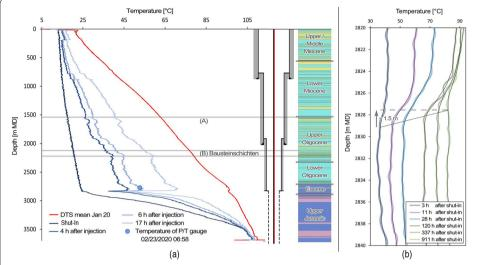
**Fig. 10** DTS profiles during warm-back of Inj2. **a** Warm-back profiles at 4, 6 and 17 h after shut-in together with the mean profile of January 2020 and the Shut-In profile over whole borehole in comparison to stratigraphic units and the well completion. **b** DTS peaks during long-term warm-back at top of the reservoir from 2810 m MD to 2840 m MD. The bold curves are raw DTS data, fine black curves are moving average over 2 m. The gray line indicates a vertical shift of about 1.5 m
