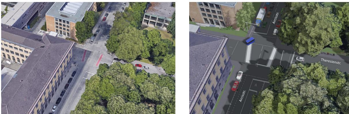
Figure 5.17: A side-by-side comparison showing Google’s illustration of the intersection on the left and the simulation systems’ environment on the right, comparing the level of detail of the digital twin.
