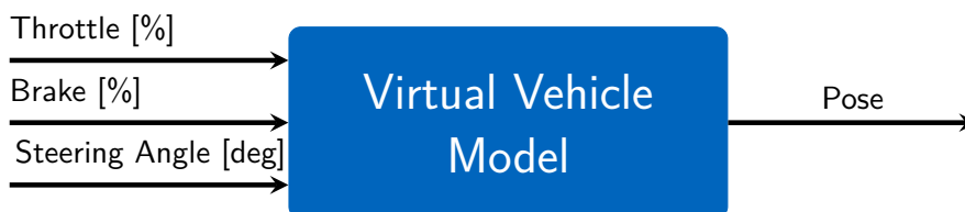
Figure 3.10: Simplified block diagram of the complete virtual vehicle model used in the simulations that utilizes throttle brake and steering angle as inputs to generate the pose as output.
