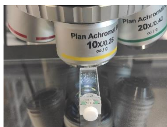
Figure 61: Experimental setup for movement observation of nanomotors.
