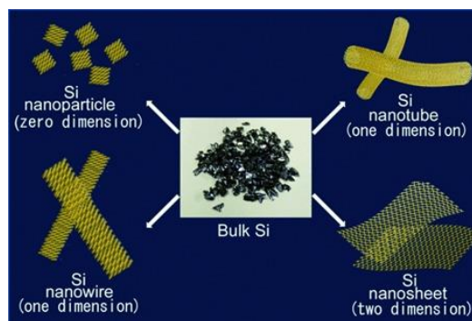
Figure 1: Schemes of different shapes and dimensions of silicon nanomaterials. Reprinted with permission from Ref. [10] .
