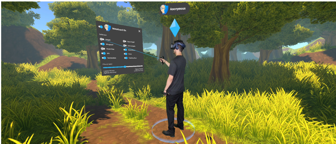
Figure 6.2.: Mixed reality photo of a user enabling “MetaGuard,” our implementation of the first proposal for a VR “incognito mode”.
