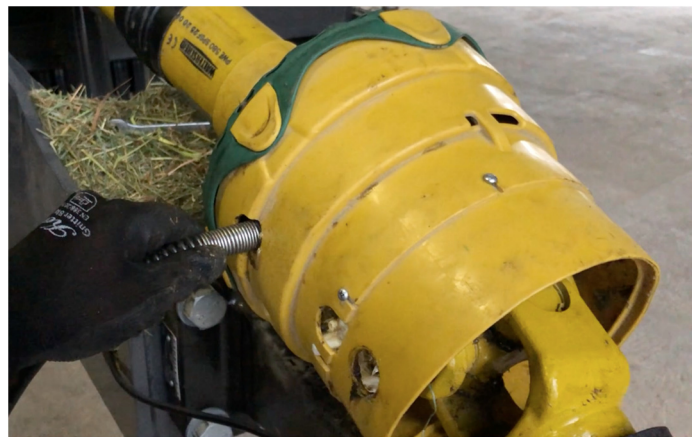
Figure 8. Lubrication through an access hole in the shaft guard of the PTO shaft [own photography].
