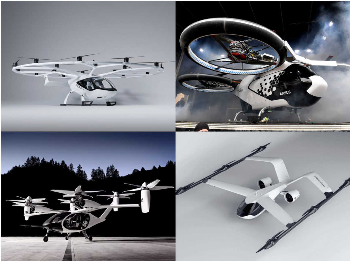
Figure 1.2: Different eVTOL Airframes. Upper Left: Volocity by Volocopter [4] - A Multirotor Configuration. Upper Right: CityAirbus by Airbus [5] - A Multirotor Configuration. Lower Left: S4 Air Taxi 2.0 by Joby Aviation [6] - A Tilt-Rotor Configuration. Lower Right: VoloConnect by Volocopter [7] - A Lift-to-Cruise Configuration with Dedicated Traction System.
