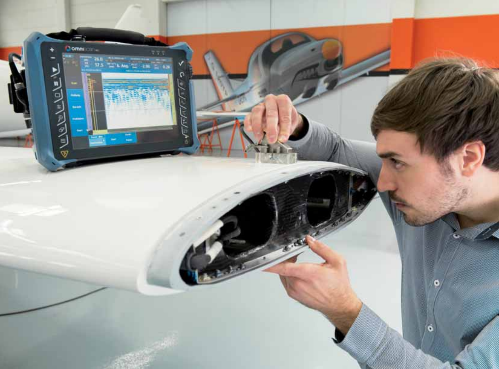
Inspection of the wing of an aircraft made of a mix of glass and carbon fiber reinforced polymers. Measurements with ultrasound phased-array sensors help in determining material structure
