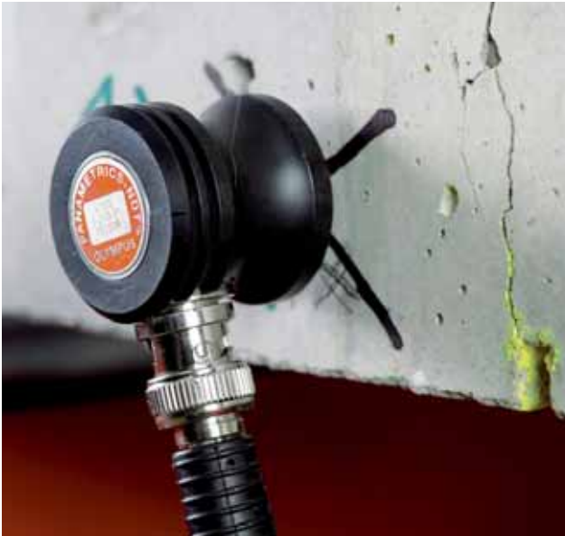
Left: Three-point bending test of concrete with self-healing capabilities. A technician prepares ultrasound sensors and sticks them onto a concrete beam containing capsules with a healing agent. The capsules break under pressure. Ultrasound and acoustic emission measurements show whether the agents are activated and all voids are properly sealed
