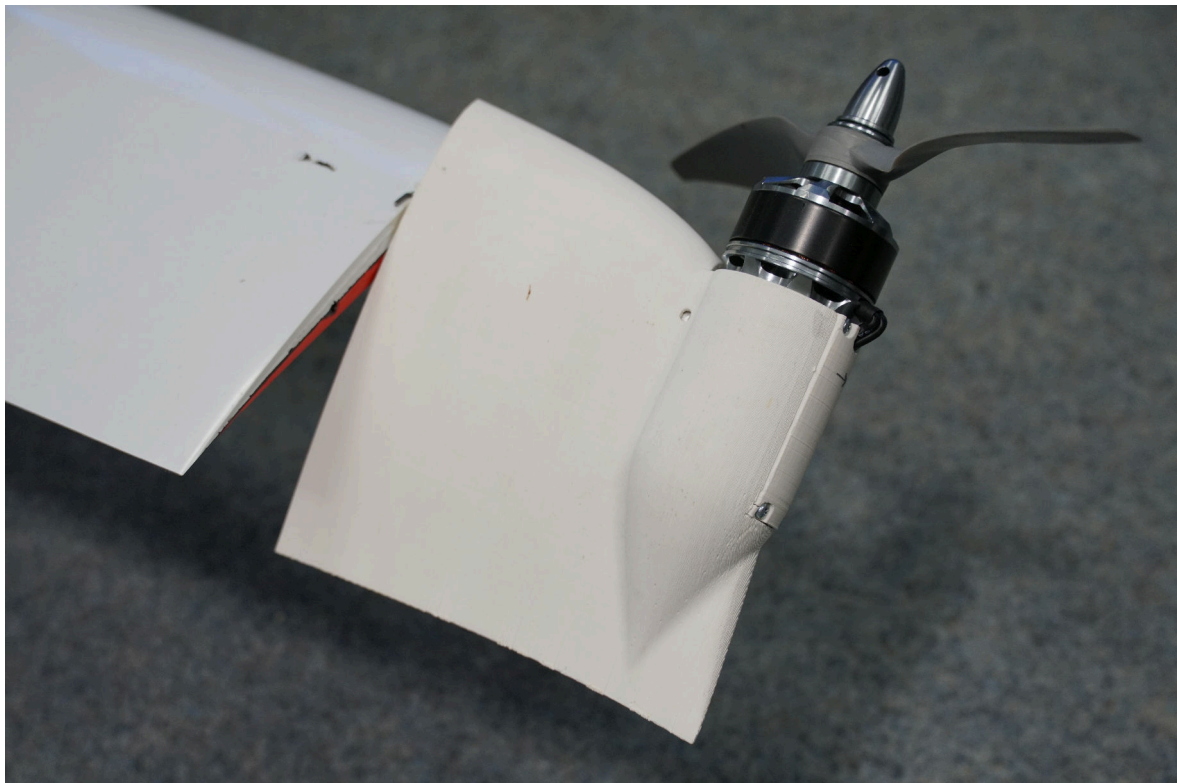
Figure 3.7: Tractor tilt wingtip of the qPt_ _tipt prototype
