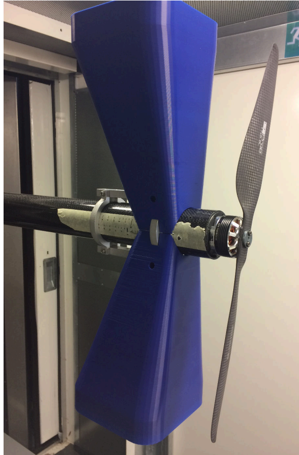
Figure 4.9: Extension to the load cell to measure rotor thrust blocking with object pyr mounted
