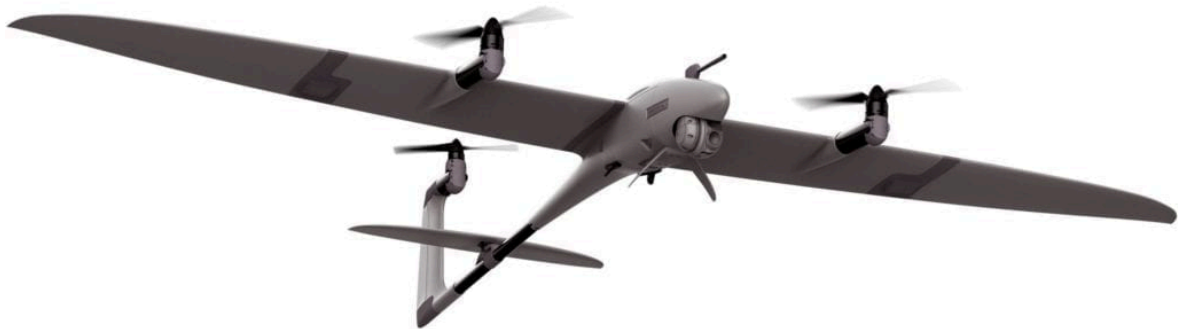
Figure 3.8: Representative of the tVt configuration: Quantum Systems Vector with powertrains in hover position
