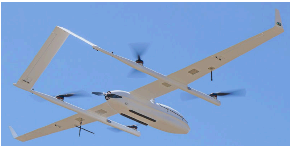
Figure 3.2: Representative of the qXc configuration: JOUAV CW-25E
