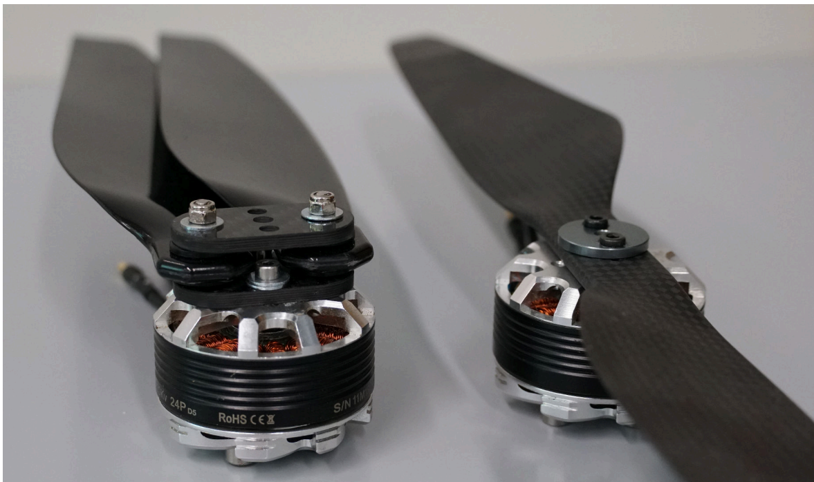
Figure 3.17: Comparison of folding rotor mount (left) and conventional rotor mount (right), both for a pusher arrangement
