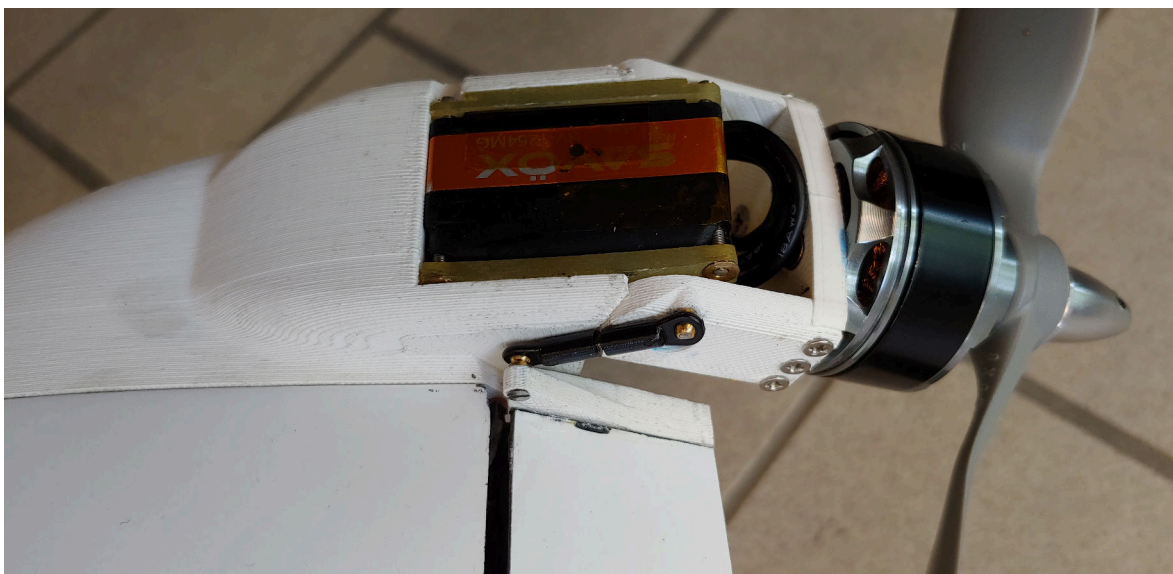
Figure 3.6: Pusher tilt powertrain of the qPt push prototype
