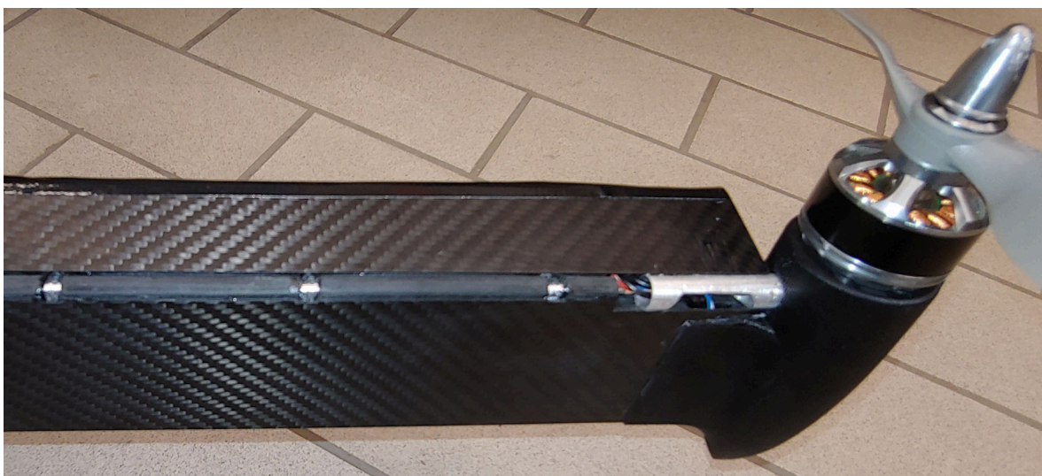
Figure 3.11: Tiltable powertrain on the horizontal tailplane of the tAt_htp prototype
