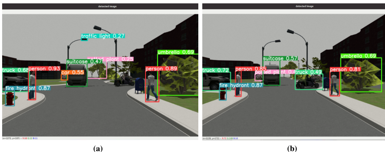
Figure 4.1 Object-detection by Yolo v5 on NRP platform (right: another frame)
