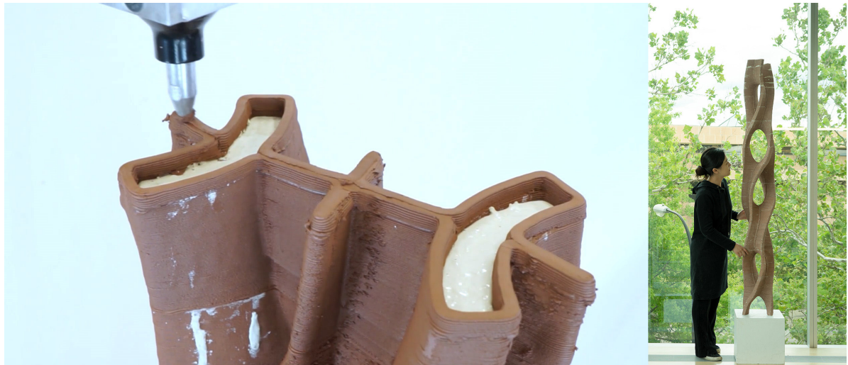
Figure 2: Incremental concrete casting process in “Cocoon” allows concrete to support the 3DP clay formwork (left). Concrete column “Cocoon” with branching geometry (right). (“Rcuxin Xie - 21SU’ Cocoon” n.d.)
