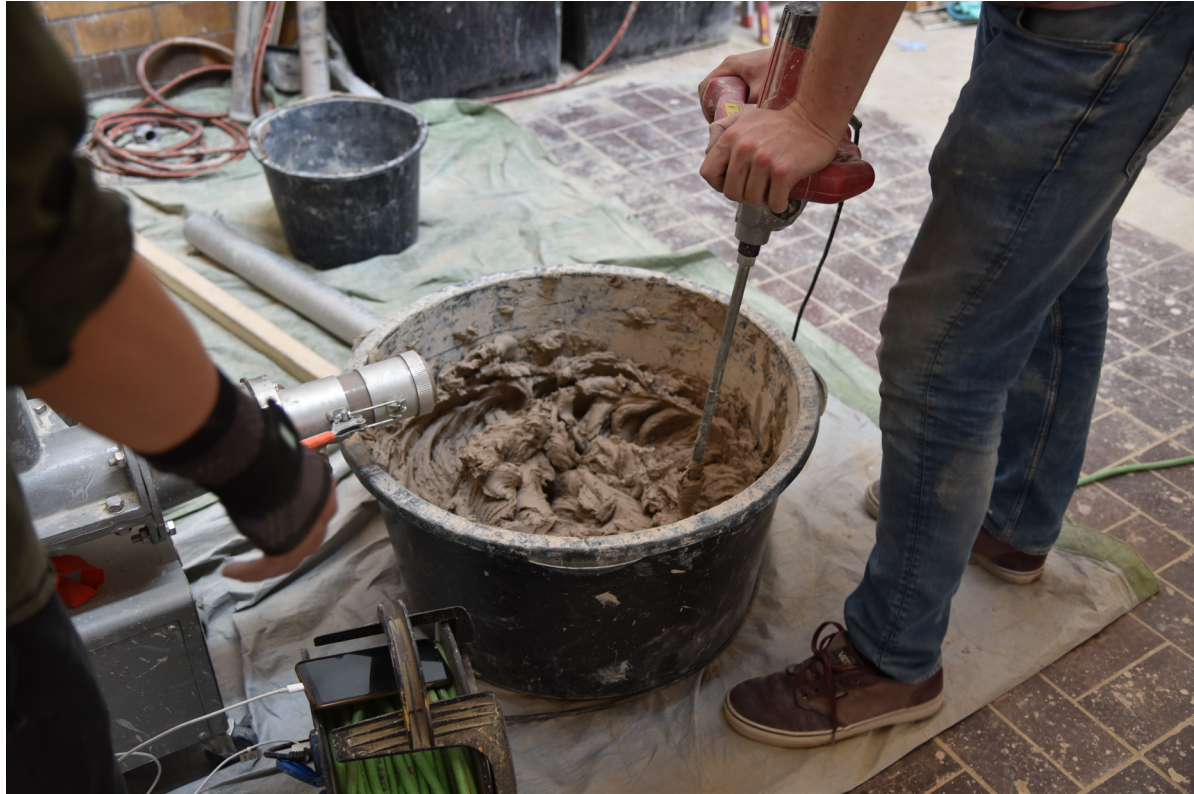
Figure 41: Clay being prepared. A bucket of clay is being mixed with water in the middle of the picture. The well-mixed clay is being filled into a cartridge with the vacuum pugmill on the left-down corner of the picture. Photo credit: Gido Dielemans
