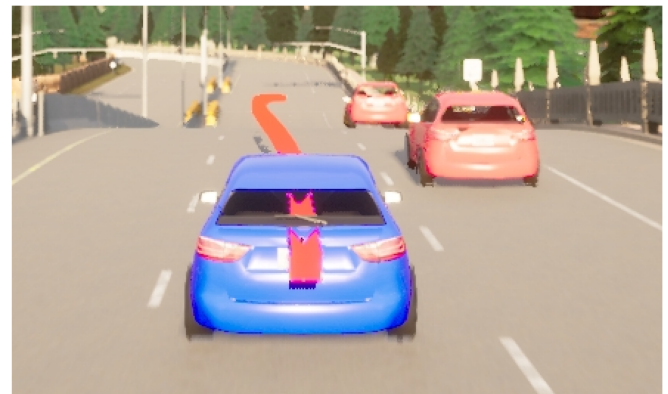
Fig. 15. Planned trajectory of the EV using the novel IMM+SMPC algorithm at time t = 4.80 s in the scenario in which TV2 eventually does not execute the lane change.
