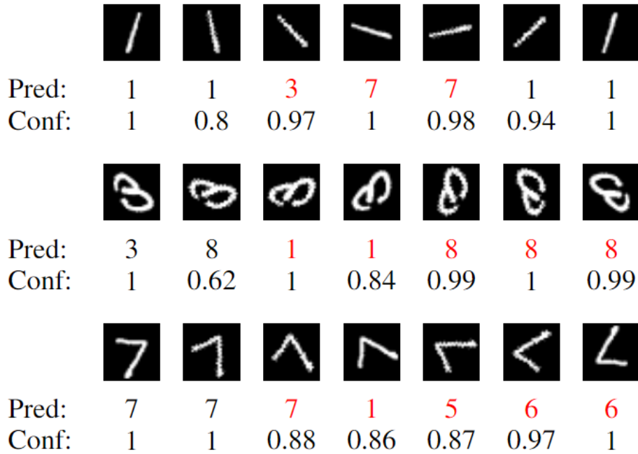
Figure 9.: Predictions obtained via a LeNet network trained on handwritten digits (from 0 to 9) of MNIST and evaluated on different rotations of test samples. For some rotations, the network exhibits a high confidence on the false class owing to confusion (e.g., 3 is confused with 8) or unknown representations. These examples show how a CNN-based classifier can generate overconfident FPs under data distribution shifts. This figure is adapted from Gawlikowski et al. [99]
