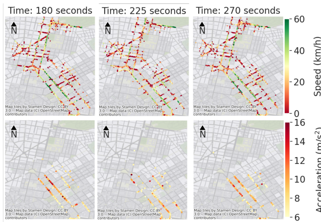
Fig. 8. Heatmap showing location-wise speeds and accelerations (exceeding 6 \text{ m/s}^2 ) at frames 45 seconds apart to highlight the correlation between them and the periodicity of excess accelerations at about 90 seconds. Similar findings were found for deceleration.
