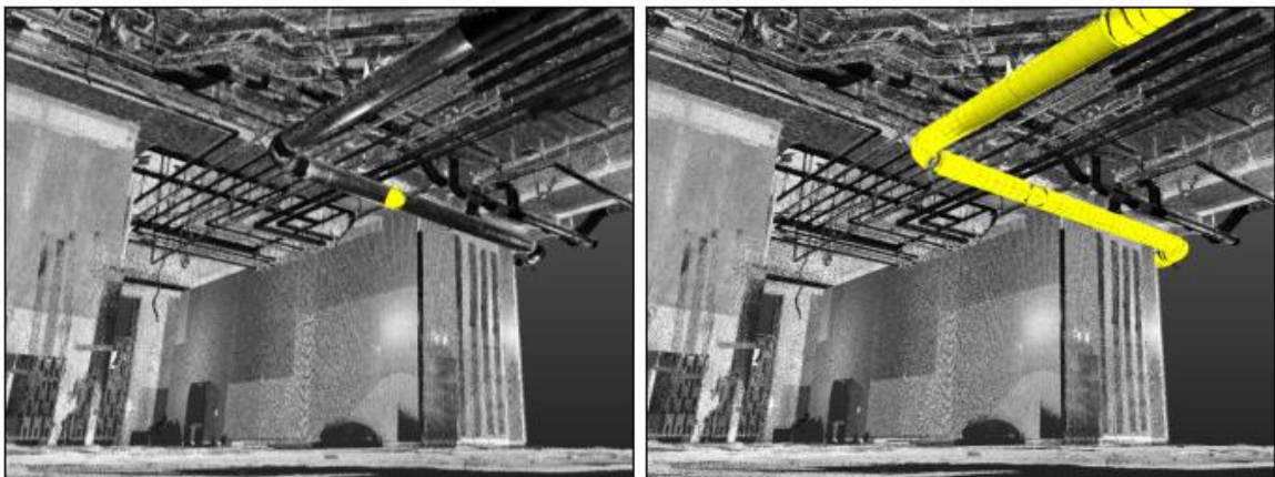
Figure 3.5 Semi-automated pipeline extraction (Son, Kim, and Turkan 2015)
