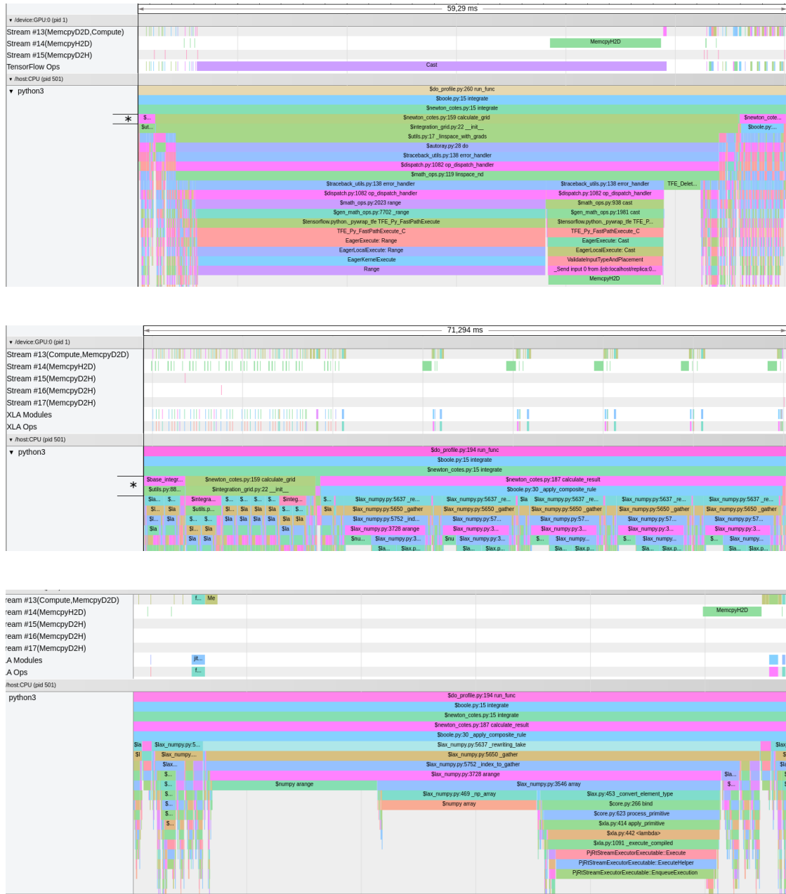
Figure 4.9: TensorBoard visualisation of collected traces with TensorFlow and JAX for a one-dimensional integrand and Composite Boole quadrature. These traces show a low utilisation of the GPU.
