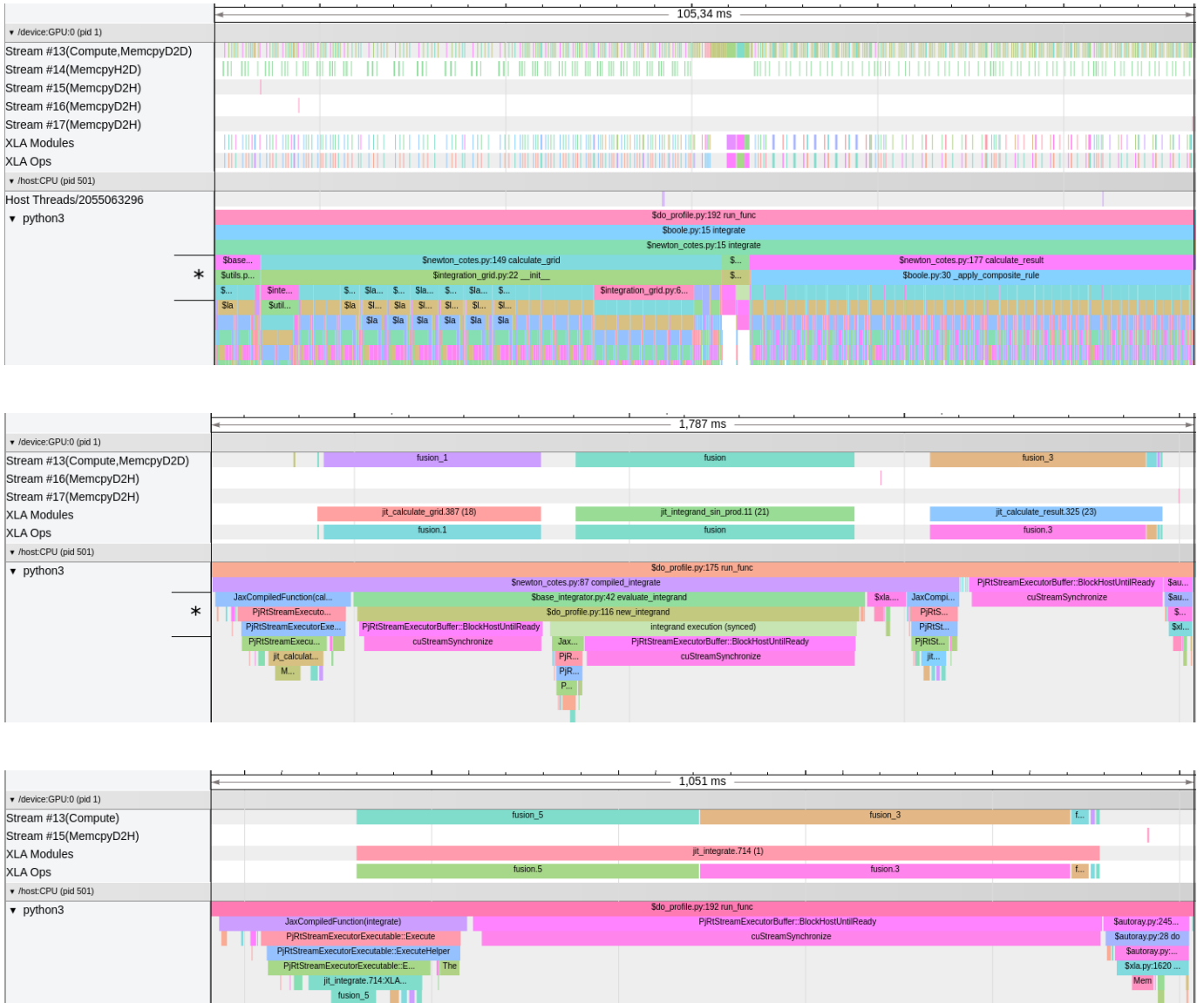
Figure 4.6: TensorBoard visualisation of collected traces with JAX and different compilations for the previously described setup. Without compilation, there are numerous small operations in the CUDA stream, and calculate_grid and calculate_result are comparatively slow. Top: Code executed in eager mode (uncompiled). Middle: Sample point calculation, integrand evaluation, and result computation separately compiled (parts compiled). Bottom: Whole integrate method compiled (all compiled)
