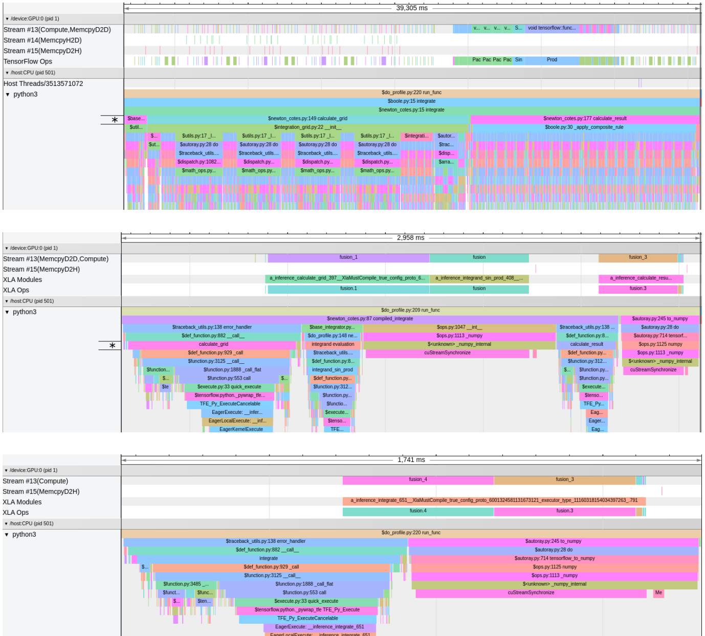
Figure 4.7: TensorBoard visualisation of collected traces with TensorFlow and different compilations for the previously described setup. Without compilation, there are numerous small operations in the CUDA stream, and calculate_grid and calculate_result are comparatively slow. Top: Code executed in eager mode (uncompiled). Middle: Sample point calculation, integrand evaluation, and result computation separately compiled (parts compiled). Bottom: Whole integrate method compiled (all compiled)
