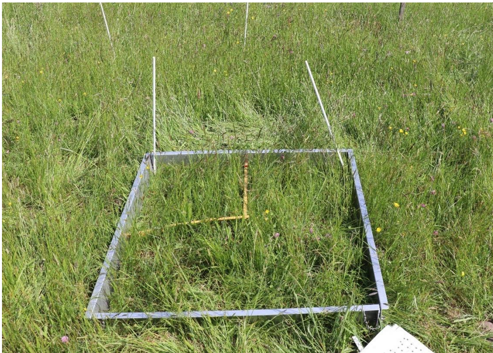
Fig. 11: A metal frame was used for counting Jacobaea aquatica plants per square metre. The white sticks mark the edges of the subplot which were marked with soil magnets.
