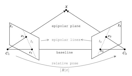
Figure 2: Epipolar geometry illustration.
