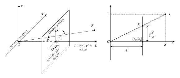
Figure 1: Pinhole camera model illustration.
