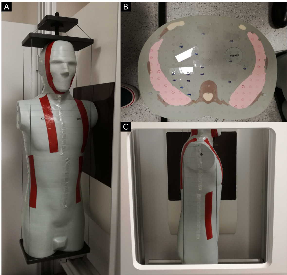
Figure 4.1: Photographs of the male anthropomorphic ATOM phantom. A, frontal view, B, cross-sectional view of one slab, and C, lateral view of phantom used to model a reference person according to ICRP 89 [Valentin, 2002] for quantitative dosimetry. In each phantom slab there are drill holes in which additional thermoluminescent dosimeters can be inserted in order to measure the locally absorbed dose at different anatomical locations. Figure adapted from [Frank, 2021].
