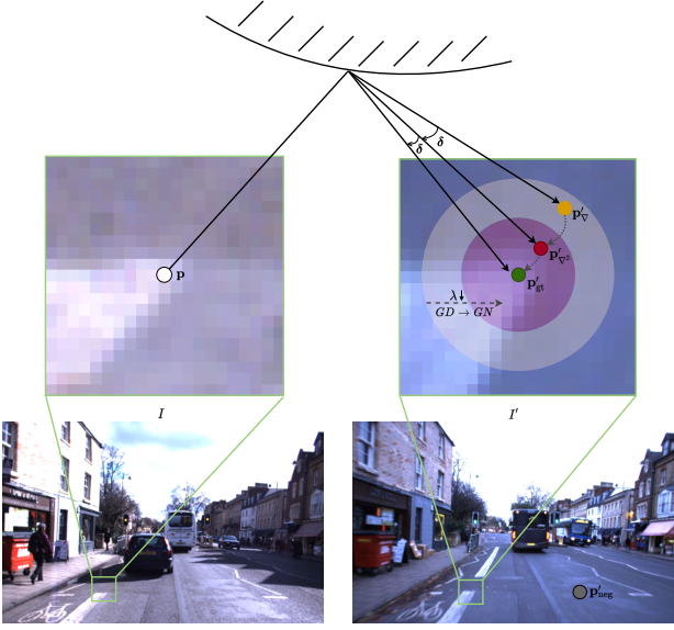
Figure 2: Visualization of the typical behavior of direct image alignment with Levenberg-Marquardt. Initially, the projected point position (orange point, \mathbf{p}'_{\nabla} ) is far away from the correct solution (green point, \mathbf{p}'_{\text{gt}} ), and \lambda is large, yielding an update step similar to gradient descent. After some iterations the projected point position gets closer to the optimum (red point, \mathbf{p}'_{\nabla 2} ) and at the same time \lambda will get smaller, leading to an update step similar to the Gauss-Newton algorithm. This is the intuition behind our point sampling strategy, where we utilize the ground-truth correspondence \mathbf{p}'_{\text{gt}} for Equation (7), a negative \mathbf{p}'_{\text{neg}} sampled across the whole image for Equation (8), a negative \mathbf{p}'_{\nabla} sampled in a far vicinity for Equation (12), and a negative \mathbf{p}'_{\nabla 2} sampled in a close vicinity for Equation (14).
