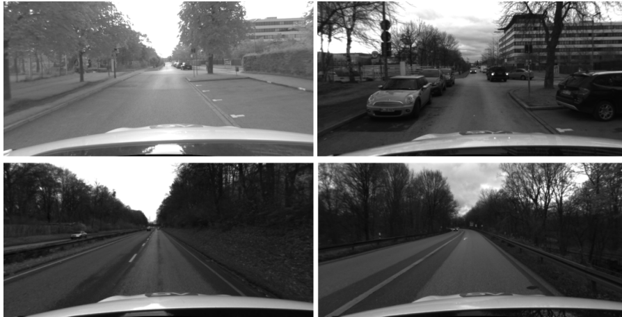
Fig. 6: Challenging scenes for global place recognition. Top: two pictures share the same location with different appearances. Bottom: two pictures have similar appearance but are taken at different locations.
