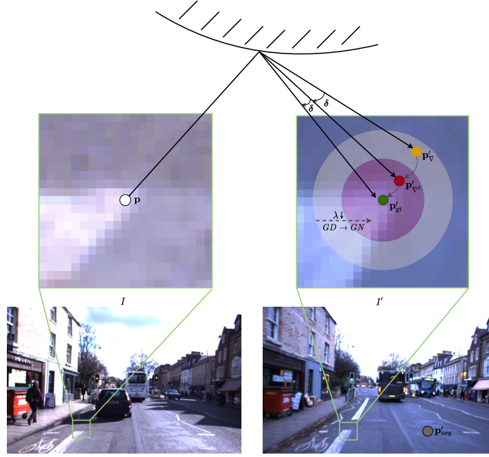
Figure 8.2: Visualization of the typical behavior of direct image alignment with Levenberg-Marquardt. Initially, the projected point position (orange point, \mathbf{p}'_{\nabla} ) is far away from the correct solution (green point, \mathbf{p}'_{\text{gt}} ), and \lambda is large, yielding an update step similar to gradient descent. After some iterations the projected point position gets closer to the optimum (red point, \mathbf{p}'_{\nabla 2} ) and at the same time \lambda will get smaller, leading to an update step similar to the Gauss-Newton algorithm. This is the intuition behind our point sampling strategy, where we utilize the ground-truth correspondence \mathbf{p}'_{\text{gt}} for Equation (8.7), a negative \mathbf{p}'_{\text{neg}} sampled across the whole image for Equation (8.8), a negative \mathbf{p}'_{\nabla} sampled in a far vicinity for Equation (8.12), and a negative \mathbf{p}'_{\nabla 2} sampled in a close vicinity for Equation (8.14).
