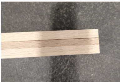
Figure 4: Discoloration of the adhesive and splitting of the glue line at the two ends of the test specimen for Adhesive 1
