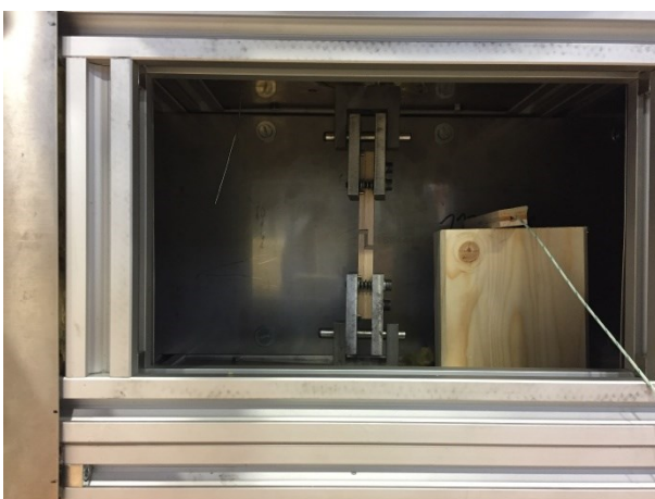
Figure 6: Temperature measurement of the glue line behind the clamping device during the creep tests under temperature load and air temperature measurement next to the clamping with a sheathed thermocouple
