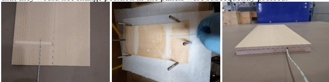
Figure 3: Inserting the thermocouples into the panel
