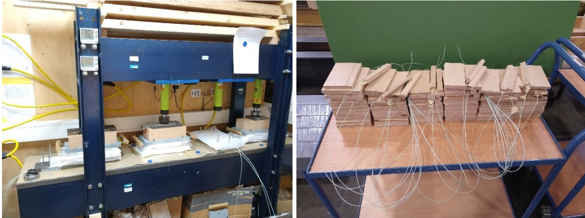
Figure 1: Left: compression of the panels; Right: Pressed and cured panels before the test specimens were cut to size
