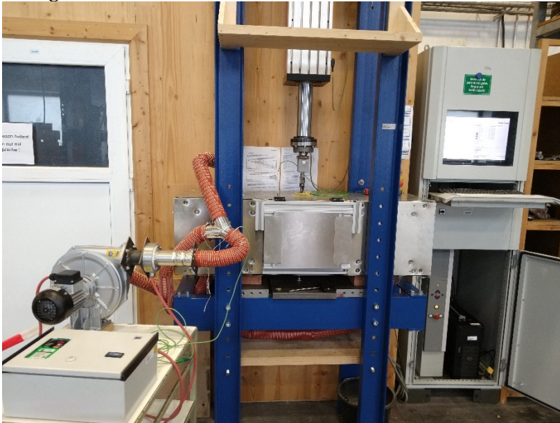
Figure 5: Built-in thermal box in test facility
