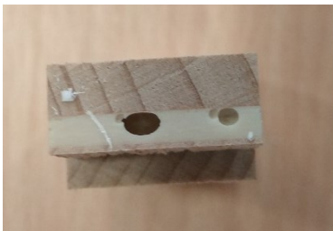
Figure 12: Bubbles in test specimens with a glue line thickness of 3.0 mm (PK 12304 48)
