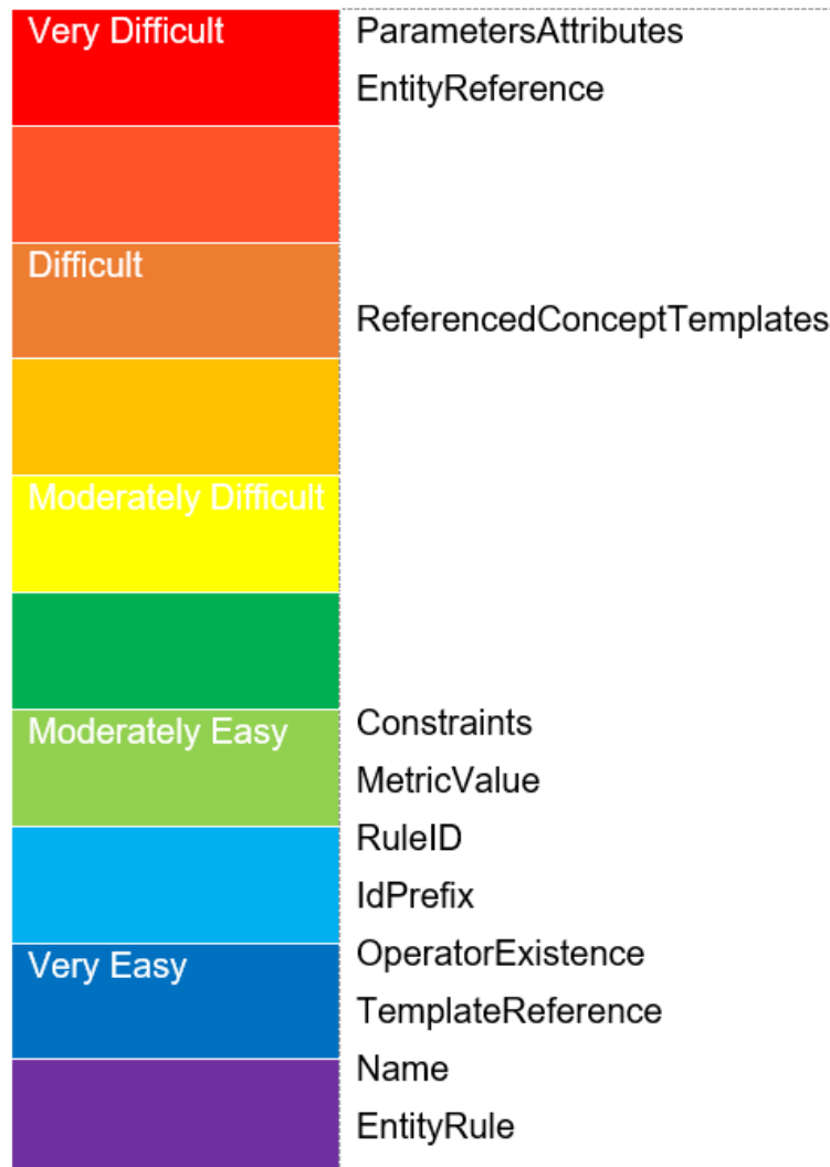
Figure 6.4: Scale of difficulty of the mvdXML checks
